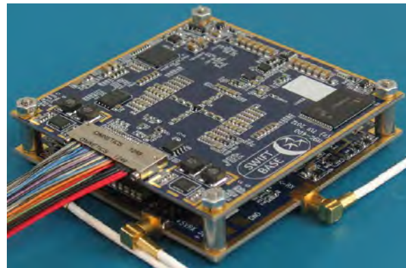
Figure 19. RelNav Radio Prototype. TUI's RelNav radio provides cross-link communications at up to 12 Mbps as well as measuring range to \leq 0.1 m and heading to \leq 1^\circ .
