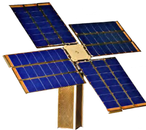
Figure 12. TUI's 'SunMill™' 80W Deployable, Steerable Array for CubeSats. Although a different solar array configuration would likely be required for NanoTHOR, the SunMill Array provides a baseline for establishing that the power requirements for NanoTHOR can be provided within 1.5 kg in mass and approximately $150K in cost.
