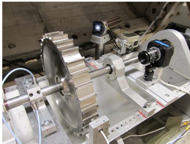
Crack Detection Experiments in GRC Rotordynamics Lab
