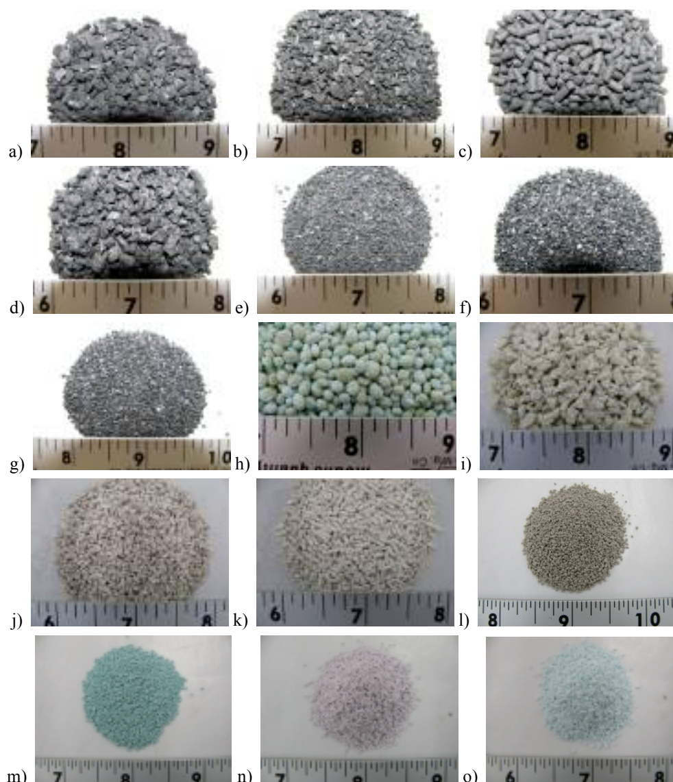
Figure 1. Materials evaluated to date for NH 3 removal capacity. a) B-S Type 3032 carbon, b) Calgon Carbon Ammosorb II, the vendor's 'replacement' carbon, c) Nucon International Ammosorb I-3, d) Tigg HP, e) 3M 6004 amine/methylamine mask cartridge, f) Molecular Products Chemsorb 1425, g) Dräger Drägercarb, h) Modern Safety Techniques LTCAT, i) Tigg KLS zeolite, j) St. Cloud natural zeolite, k) UOP HISIV 3000. l) Co-X zeolite m) Cu-X zeolite n) Co-Y zeolite o) Cu-Y zeolite. Scale markers in inches.
