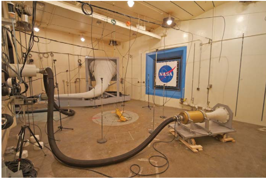
Figure 2: Photograph of SALT reverberant room shown configured for high-intensity acoustic testing with airstream modulators coupled to 35 Hz (large) and 160 Hz (small) horns.
