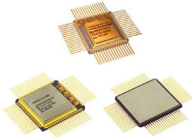
Figure 3.3-1. Honeywell 1-Mb (top) and 16-Mb (bottom-left and bottom-right) MRAM. Bottom-right image shows mu-metal magnetic shielding on bottom of package (this is the case for both 1_Mb and 16_Mb) [18].
