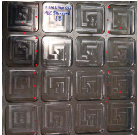
(b) FGB wall with manufactured flaws (red dots on left side are EDM notch locations; red dots on right side are partial through-the-wall hole locations)
