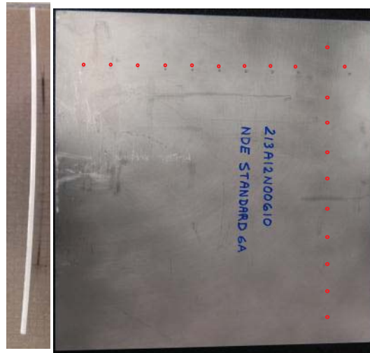
Figure 7.1-7. Standard 6A, which has the Same Manufactured Flaw Pattern as Created in Standard 2 (red dots on right side are EDM notch locations, and red dots along the topside are partial through-the-wall hole locations; Standard 6B is the same size, except that the EDM notches and partial through-the-thickness hole locations are transposed; the photo on the left side indicates the curvature of the plate)
