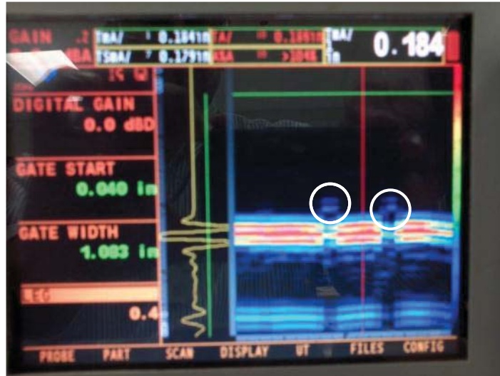
Figure 7.1-35. A B-scan Image of Impact Test Plate 1907 showing the Results of Imaging the Pits Through-the-Thickness of the Plate without a Repair Patch
