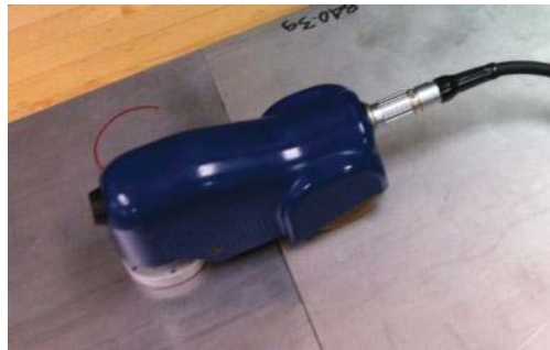
Figure 7.2-4. Large EC Probe (wheel encoder is housed in the blue casing)
