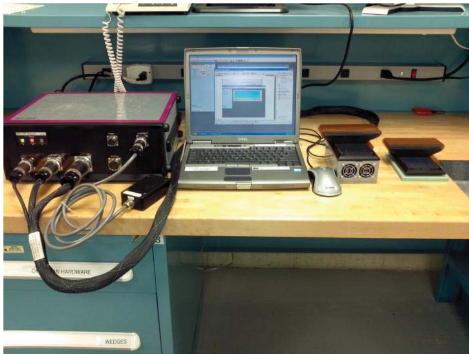
Figure 7.1-43. Jentek GridStation MWM System
