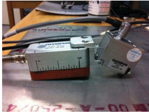
Figure 7.2-3. Large EC Probe with Mechanical Wheel Encoder
