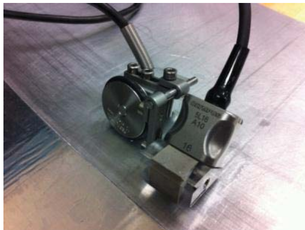
Figure 7.2-2. Ultrasound Array with Mechanical Wheel Encoder
