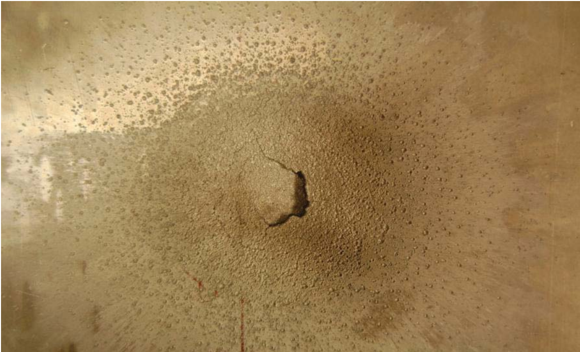
Figure 7.1-10. Backside of Impact Plate 1900, a 1/8-inch-thick Panel (this plate shows major cracking at the plate's center; the whole center region is deformed, pushing away from the backside; and there is extensive pitting around the center regions)
