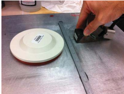
Figure 7.2-1. Scanning using a Metal Ruler as a Guide
