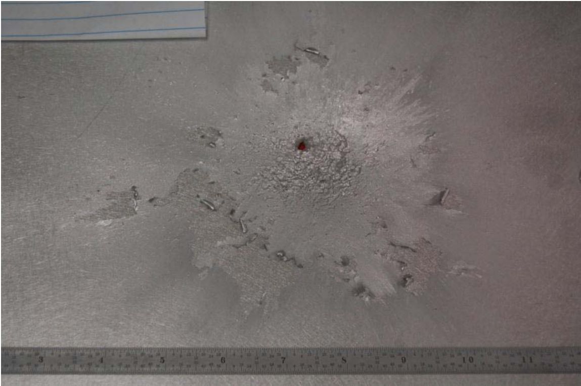
Figure 7.1-9. Backside of Impact Plate 186 (this plate shows one visible penetration, a region of deformation of the plate, and a small area of pitting)
