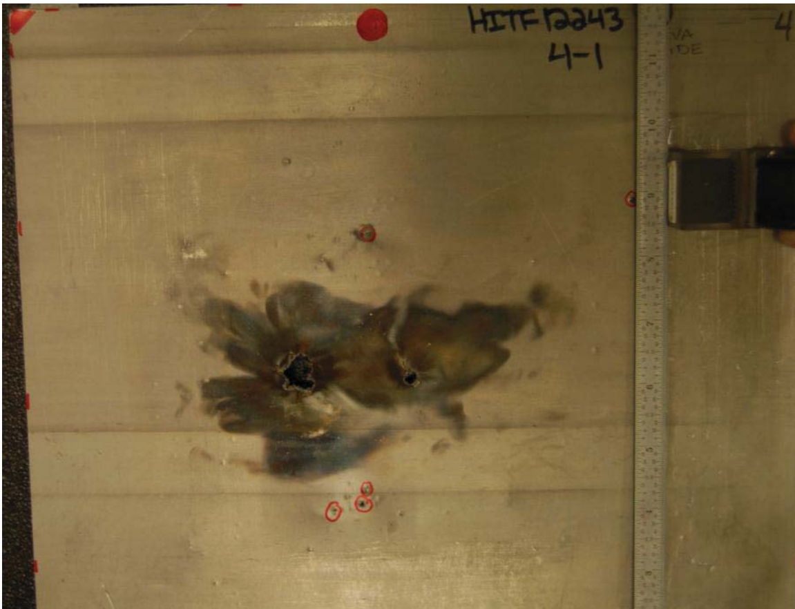
Figure 7.1-13. Backside of Impact Plate 243, which Represents FGB Wall and was Impacted with a Hypervelocity Projectile (the impact was performed from the waffled side of the plate; because of the thin wall, there are many small penetrations, some of which are highlighted in red, as well as two major penetrations; this plate shows major pitting near the center of the plate, and a few larger pits are penetrations through the plate; the areas in between the waffle walls show deformation)
