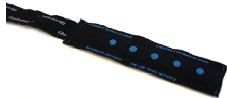
Figure 5. Fibretronics Lite Keypad these are the buttons integrated into the button forearm sleeve
