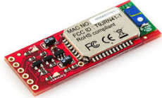
Figure 3. Bluetooth device This chip is used in the accelerometer forearm sleeve
