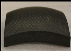
Post Arcjet Tested Coupons Resin Infiltrated
