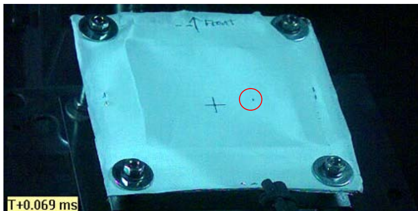
Figure C.30: Test #14 Phantom v711 high speed video image of projectile prior to impact
