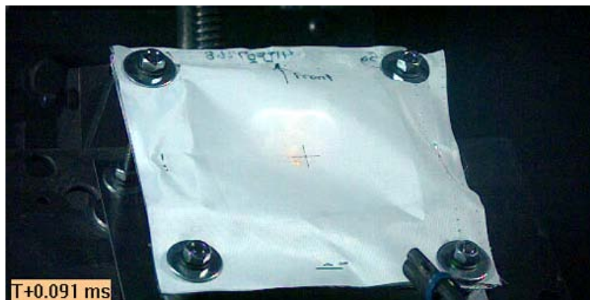
Figure C.38: Phantom v711 video image of projectile impacting Test #15C article
