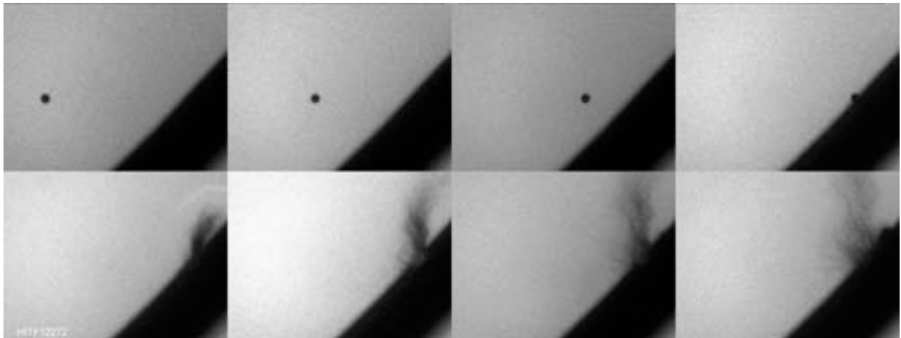
Figure C.22: High speed video of projectile in flight on Soyuz OM Test #12 using SIMX-8 High Speed Video Camera
