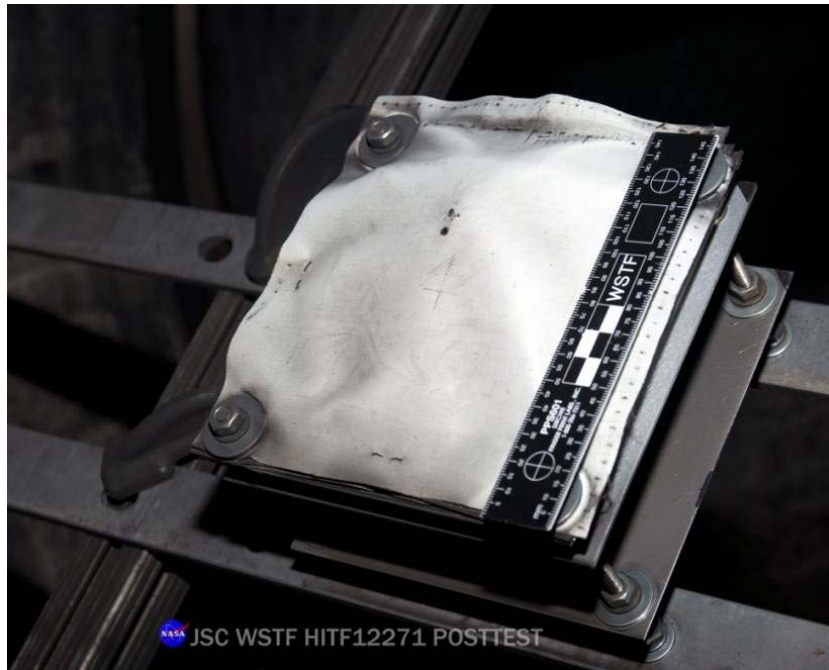
Figure 180: Post-test of ISS Soyuz Orbital Module Test #11 (HITF12271) article mounted in 0.50-caliber target tank.
