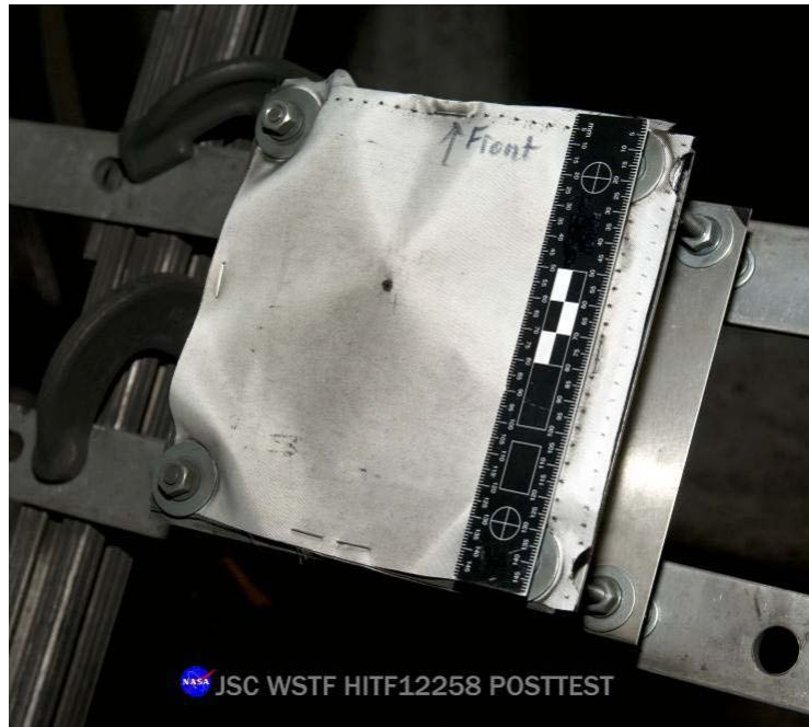
Figure 33: Post-test of ISS Soyuz Orbital Module Test #2 (HITF12258) article mounted in 0.50-caliber target tank.
