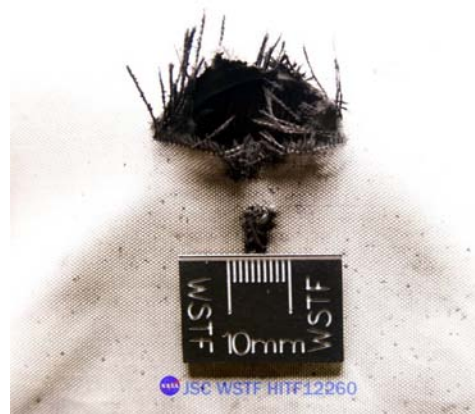
Figure 70: Beta Cloth Bumper of ISS Soyuz Orbital Module Test #4
