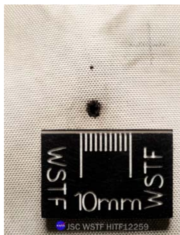
Figure 53: Beta Cloth Bumper of ISS Soyuz Orbital Module Test #3
