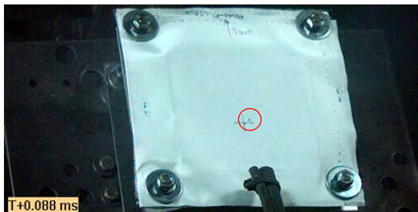
Figure C.43: Phantom v711 high speed video image of projectile prior to impact
