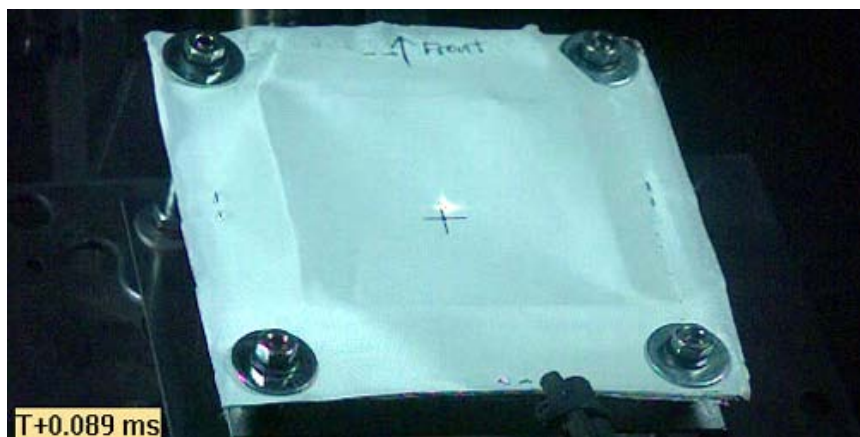
Figure C.31: Phantom v711 video image of projectile impacting Test #14 article
