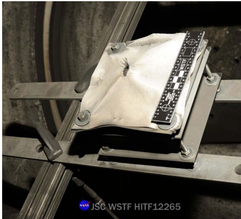
Figure 147: Post-test of ISS Soyuz Orbital Module Test #9 (HITF12265) article mounted in 0.50-caliber target tank.
