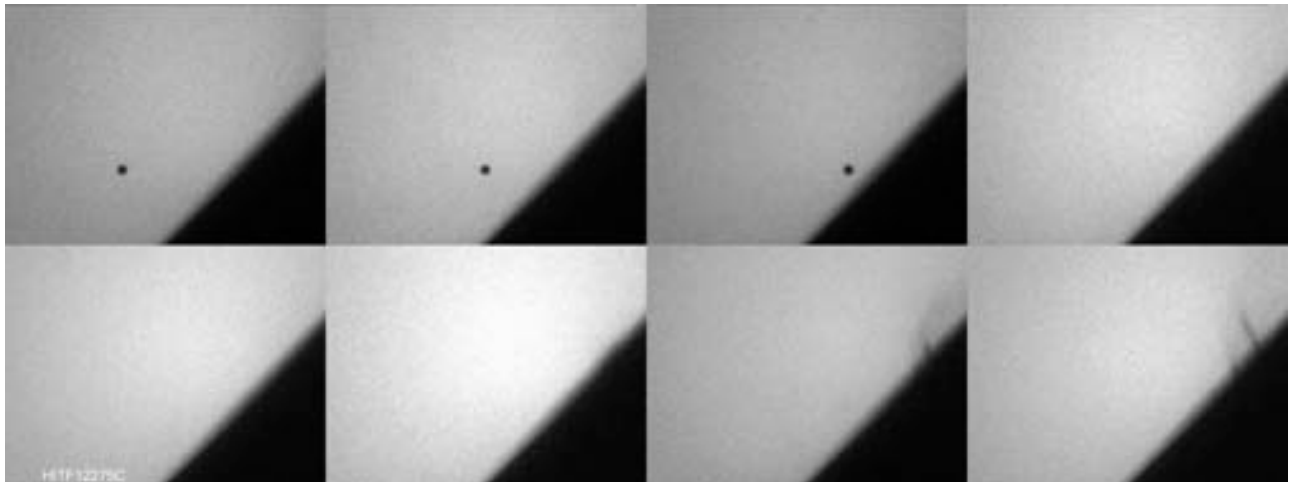
Figure C.36: High speed video of projectile in flight on Soyuz OM Test #15C using SIMX-8 High Speed Video Camera
