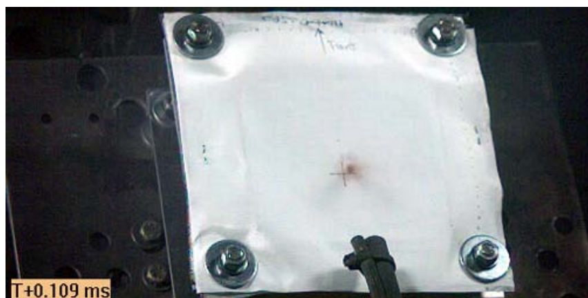
Figure C.44: Phantom v711 video image of projectile impacting Test #17 article
