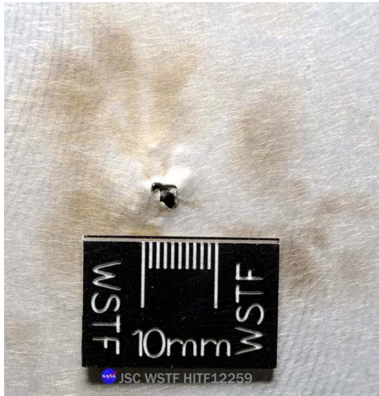
Figure 65: Al 5456-0 Rear Wall (Back) for ISS Soyuz Orbital Module Test #3
