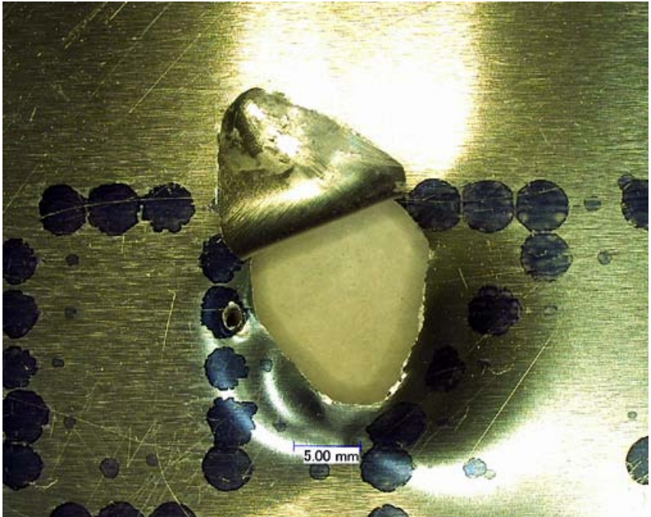
Figure 93: Al 6061-T6 Layer 7 Back of ISS Soyuz OM Test #5 (Keyence 3D Microscope Image)
