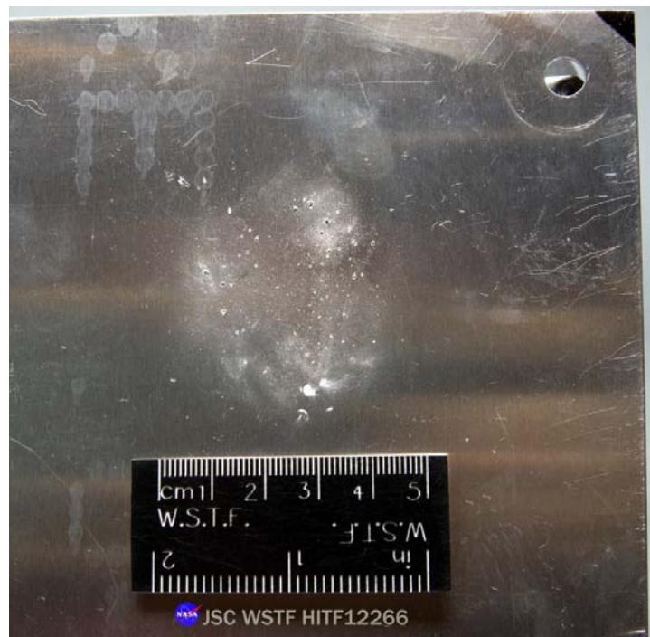
Figure 179: Front Witness Plate View of ISS Soyuz Orbital Module Test #10
