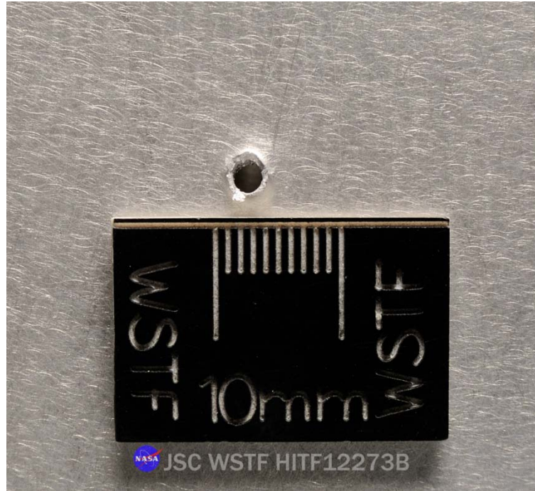
Figure 230: Al 5456-0 Rear Wall (Back) for ISS Soyuz Orbital Module Test #13B
