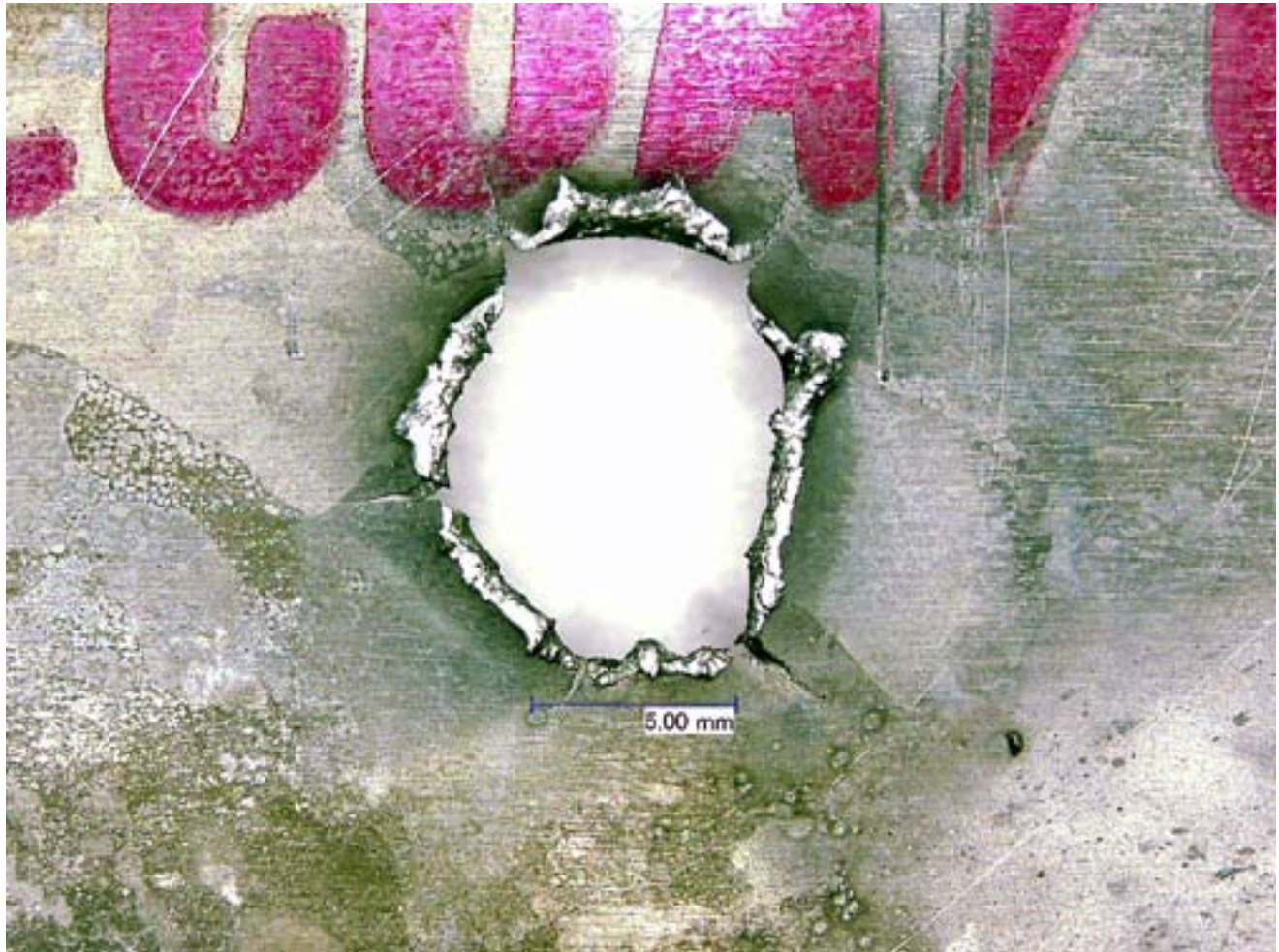
Figure 25: Al 6061-T6 Layer 7 Back of ISS Soyuz OM Test #1 (Keyence 3D Microscope Image)
