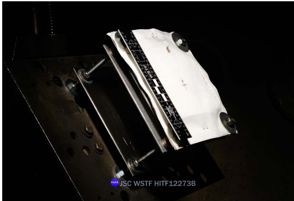
Figure 214: Post-test of ISS Soyuz Orbital Module Test #13B (HITF12273) article mounted in 0.17-caliber target tank.
