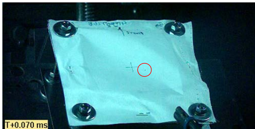
Figure C.37: Test #15C Phantom v711 high speed video image of projectile prior to impact
