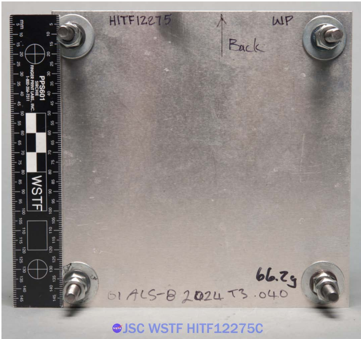
Figure 263: Back Witness Plate View of ISS Soyuz Orbital Module Test #15C
