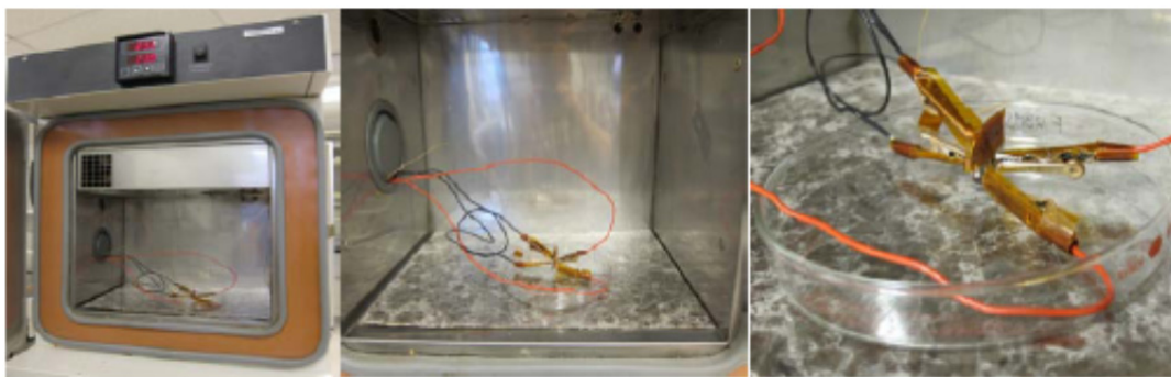
Figure 7.—A wired coin cell test fixture within the Tenny environmental chamber.
