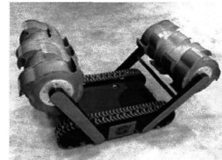
RASSOR (Regolith Advanced Surface Systems Operations Robot) will feed the hoppers
