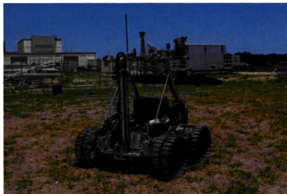
Figure 2. RESOLVE Moon Rover Field Test Unit. The LAVA subsystem is depicted in the black box on the rover. Photo credit: NASA/Dmitri Gerondidakis
