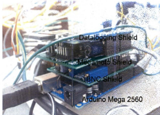
Figure 1. Setup of the Arduino Shields
