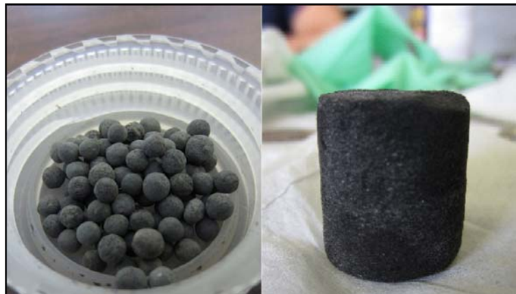
Figure 1. Pelletized (left) and Substrate (right) catalysts.
