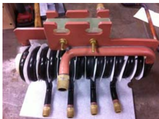
Induction Coil without Insulation
