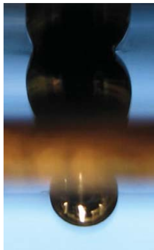
Fig. 25 Gallium capillary bridge demonstrated on copper substrates and removed from experimental apparatus.
