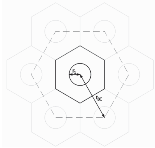
Fig. 13 Schematic of the periodic hexagonal areas associated with staggered arrays.
