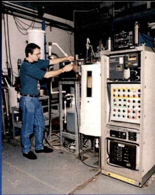
Solid Waste Stirred Tank Reactors
