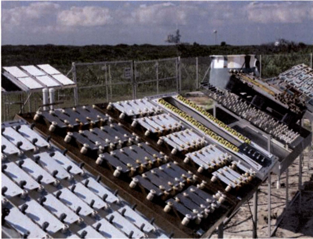
Figure 5: Test panels at KSC Beachside Atmospheric Test Facility
