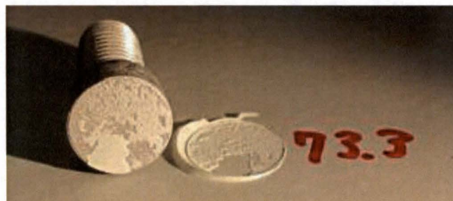
Figure 4: Typical epoxy failure while coating remained intact
