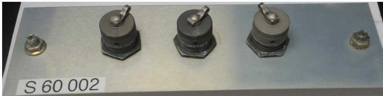
6061-T6 test panels following 35 days of ambient office storage
