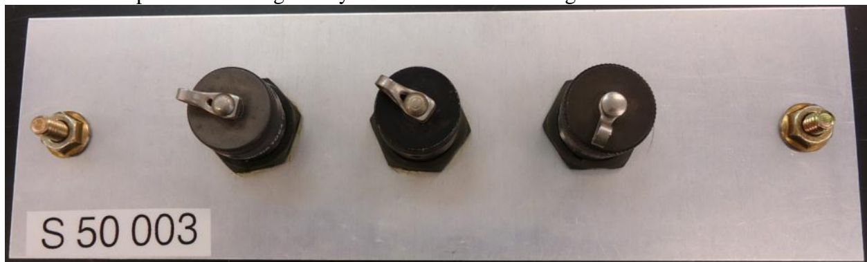
5052-H32 test panels following 70 days of ambient office storage
