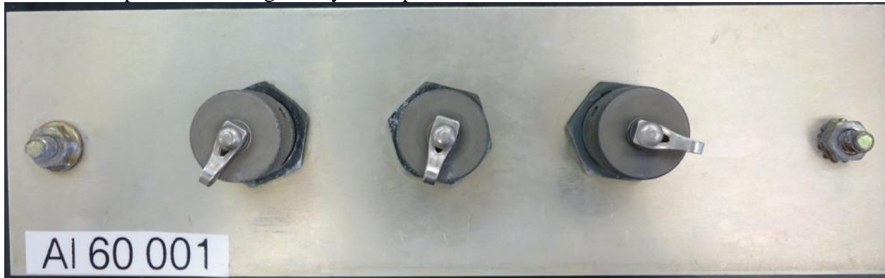
6061-T6 test panels following 70 days of exposure at the KSC Beachfront
