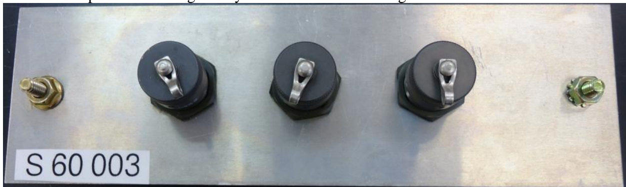
6061-T6 test panels following 70 days of ambient office storage
