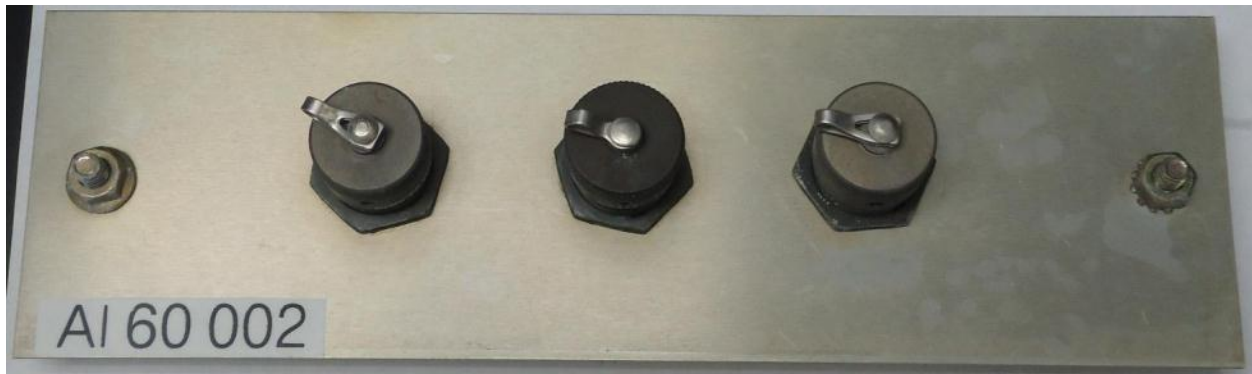
6061-T6 test panels following 35 days of ambient office storage
