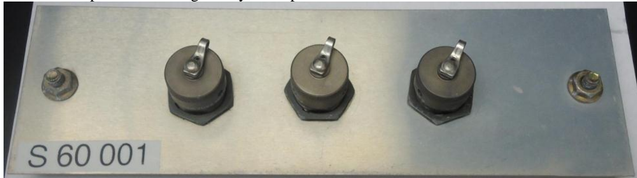
6061-T6 test panels following 35 days of exposure at the KSC Beachfront
