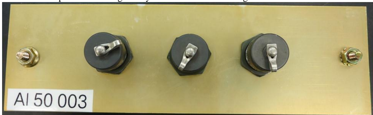
5052-H32 test panels following 70 days of ambient office storage
