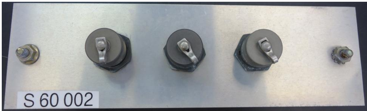
6061-T6 test panels following 70 days of ambient office storage
