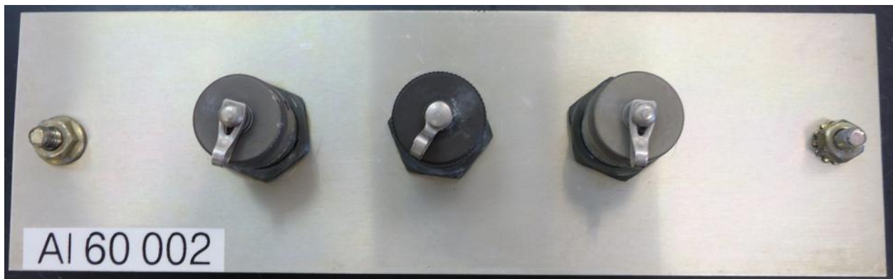
6061-T6 test panels following 70 days of ambient office storage
