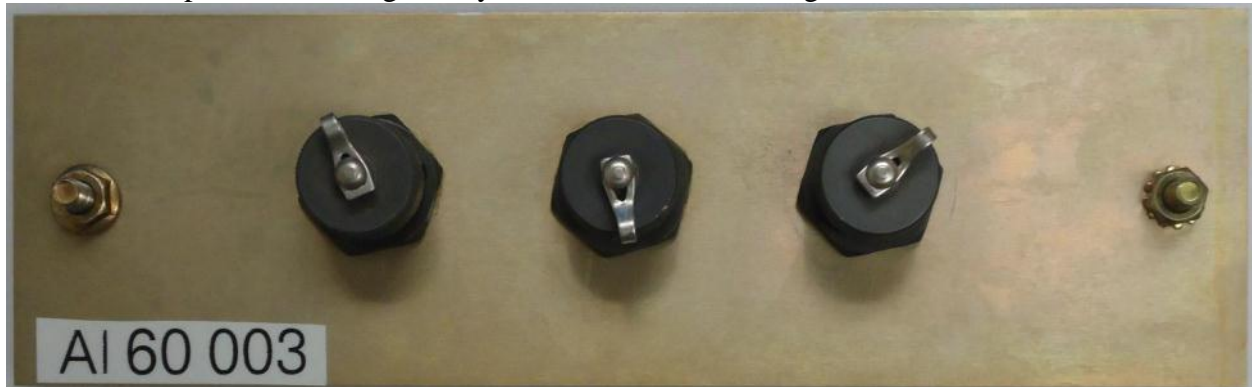
6061-T6 test panels following 35 days of ambient office storage
