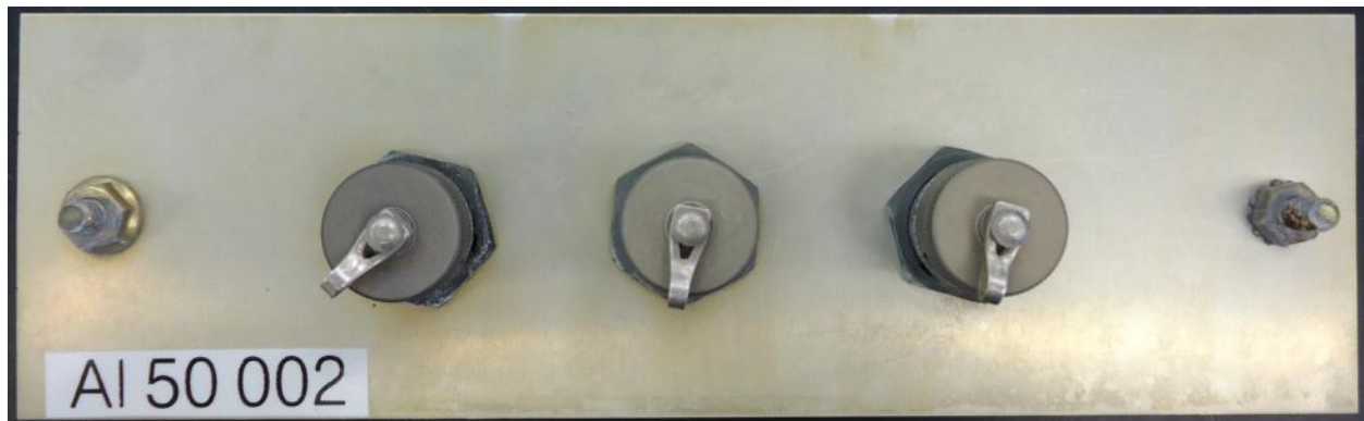
5052-H32 test panels following 70 days of ambient office storage
