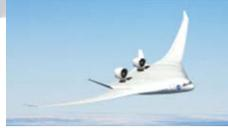
GC3 MDAO of a highly-flexible advanced aircraft configuration
