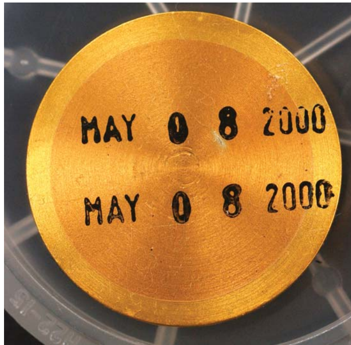
Figure 19. Ink stamp with clear overcoat from MISSE-1 ram-facing side.
