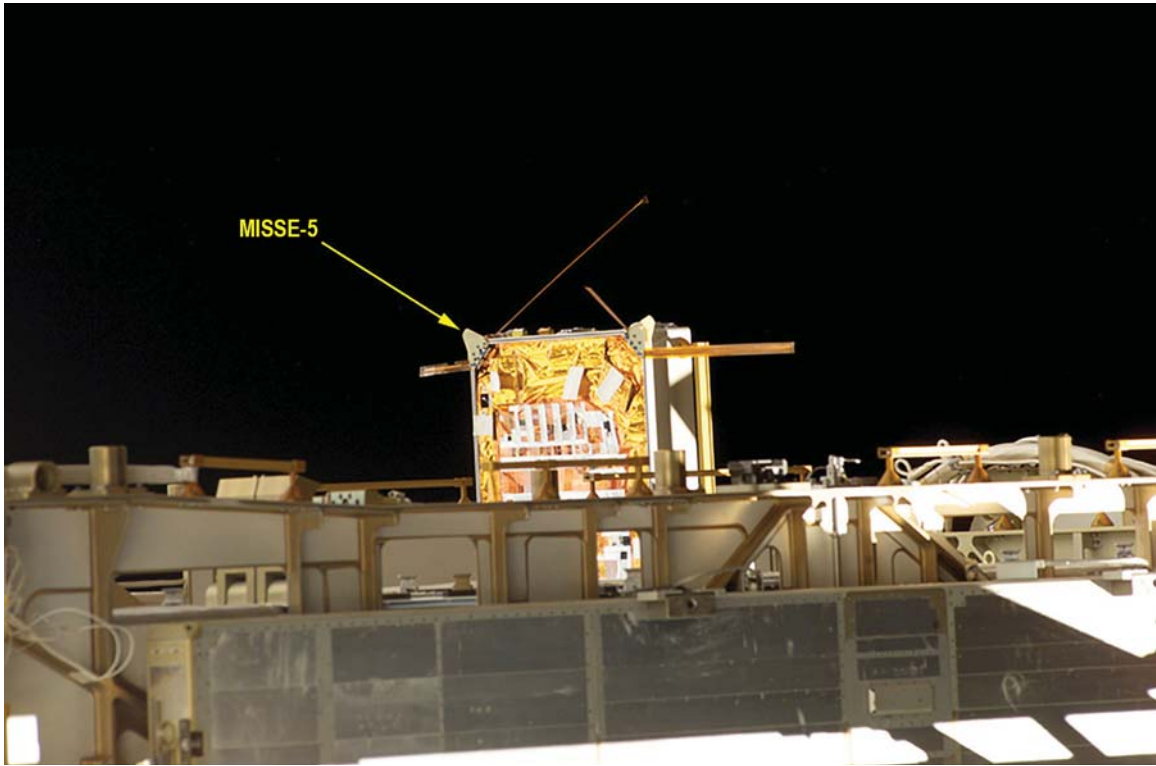
Figure 3. MISSE-5 on P6 truss; nadir side visible.
