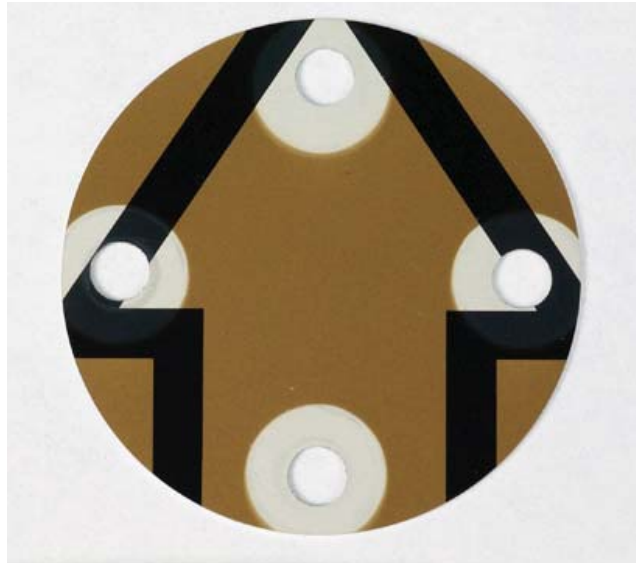
Figure 18. Metalphoto/Photofoil from MISSE-1 wake-facing side. White circles are where washers protected the surface from UV radiation.
