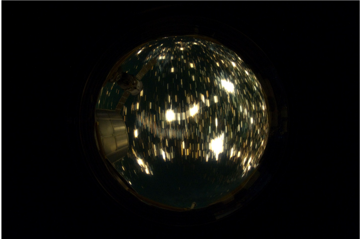
Figure 3 – View from the ISS nadir camera during Orbit 2 (over Texas). A Nikon D3S DSLR camera with 8mm f/2.8 lens was used with an exposure time of 5 s. The observing area is much reduced from that in Figures 2.
