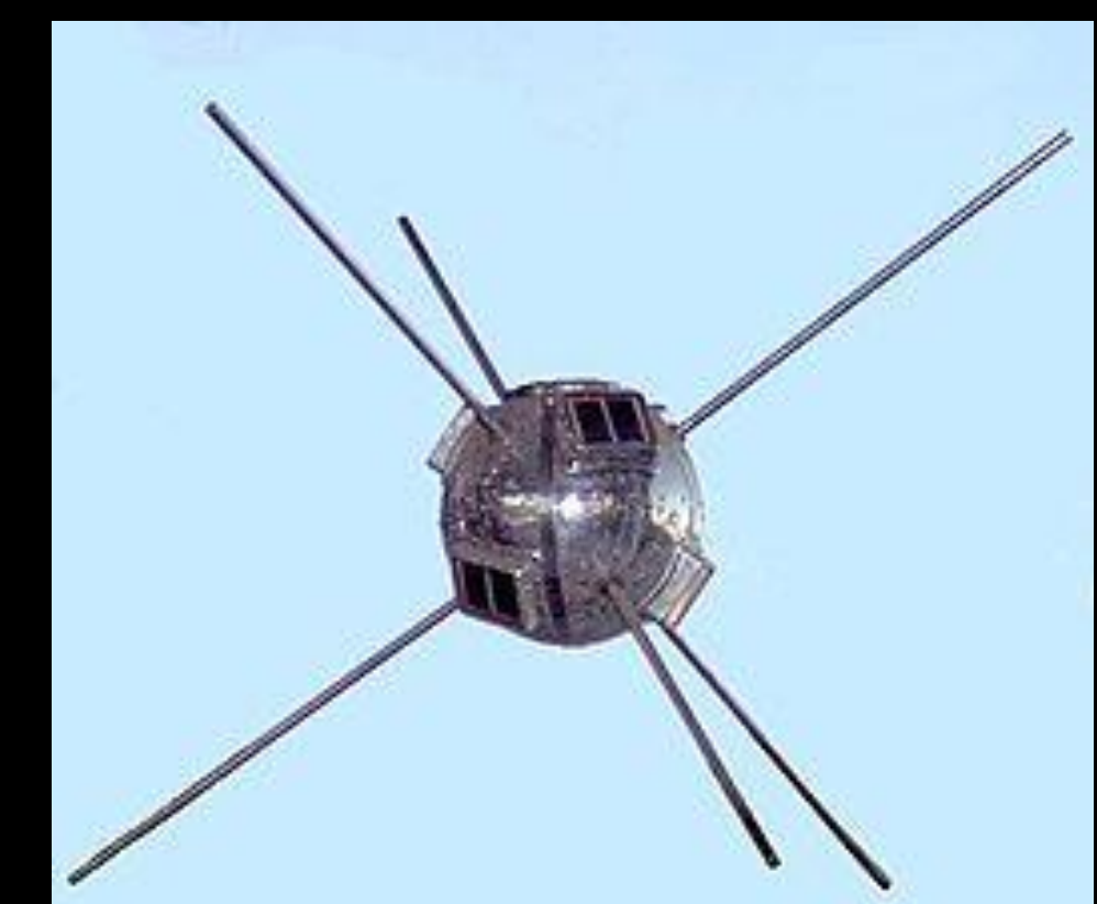
Vanguard I, launched in 1958, was the first spacecraft that used solar panels. The arrays had a 14% terrestrial efficiency.
