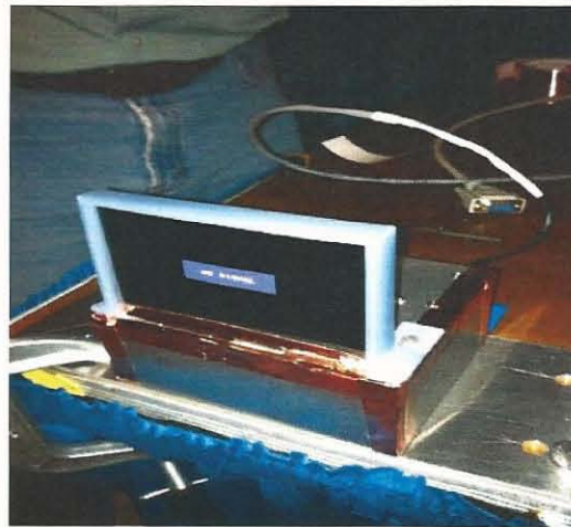
Figure 6 AMOLED #1 Mounted to the EMI Test Table
