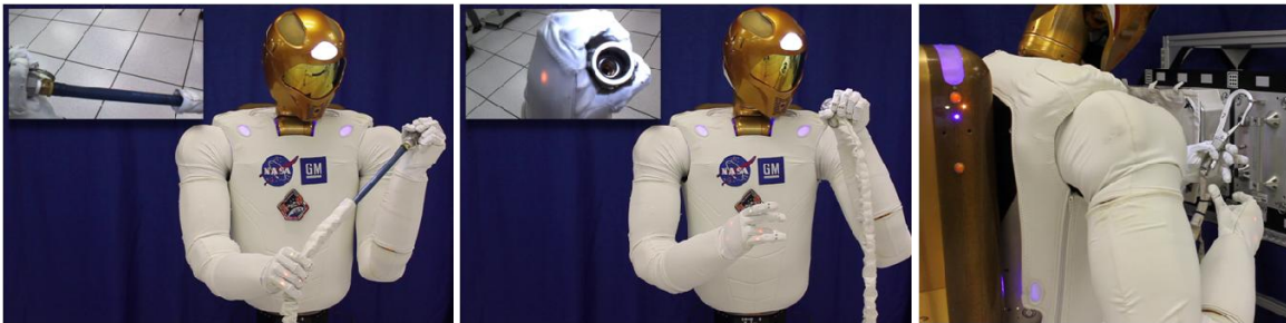
Figure 2: R2 working with EVA hoses and a tether hook.
