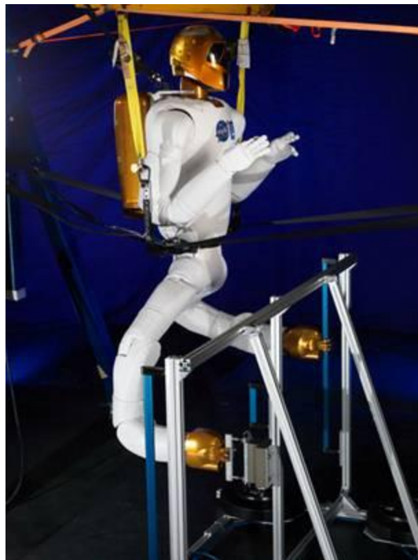
Figure 1: R2 climbing across IVA handrails during ground testing
