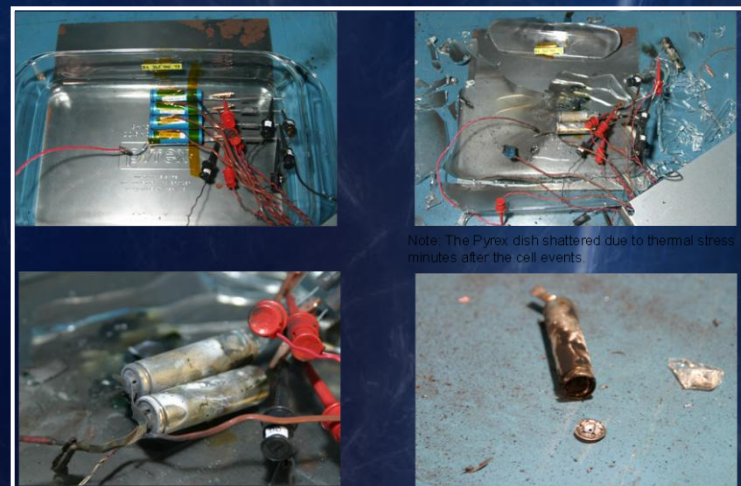
12V 6A Overcharge on 4P Battery
