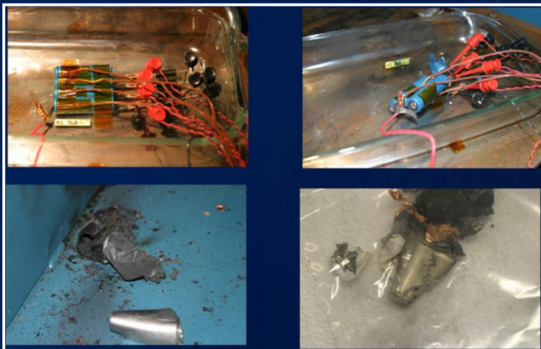
48V 6A Overcharge on 4P Battery
