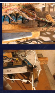
Overcharge Test on a 14-Cell String
