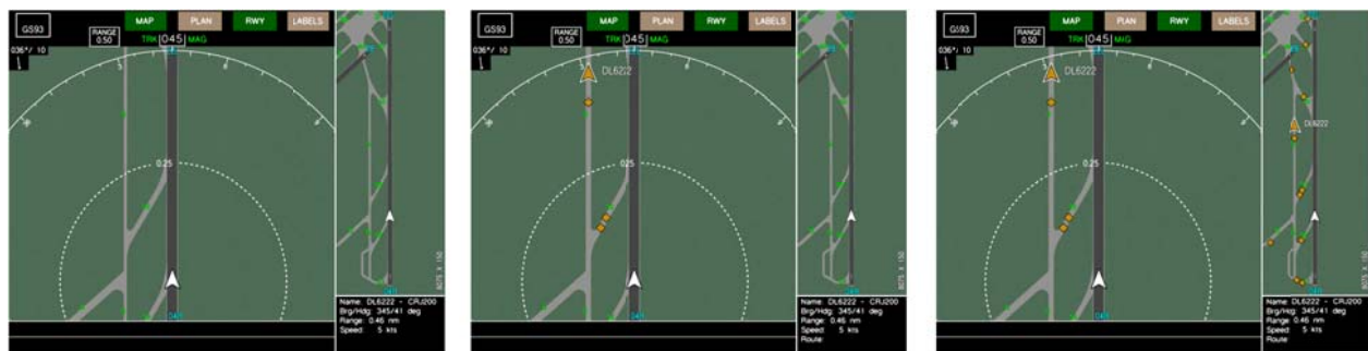
Figure 8. CDTI formats – None (left), Moving Map (center), and Moving Map/Runway Inset (right)
