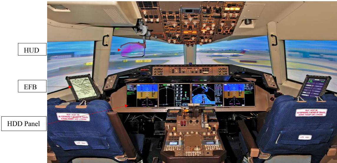
Figure 1. Research Flight Deck Simulator with HUD, Head-down Instrument Panel, and EFB
