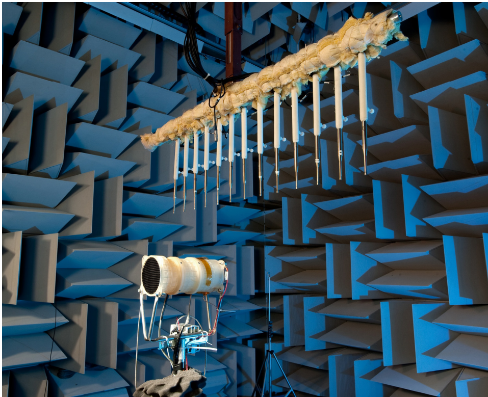
Figure 3.—Photo of the linear traverse array suspended from 3-D traverse.
