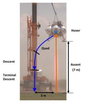
Figure 5 – Ground Take-off And Landing (GTAL) Profile
