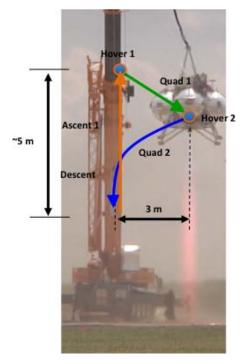
Figure 11 – Tether Test 30, 31, and 32 Profile
