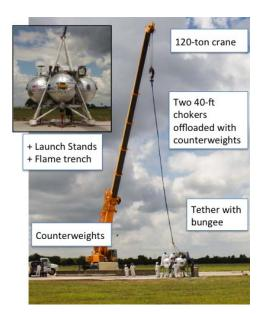
Figure 4 – Ground Take-off And Landing (GTAL) Test Configuration
