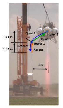
Figure 10 – Tether Test 28 and 29 Profile
