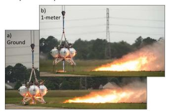
Figure 8 – Morpheus Hot-Fire 9 (HF9) Test Firings a) Ground Hot-Fire b) Low-Altitude Hot-Fire
