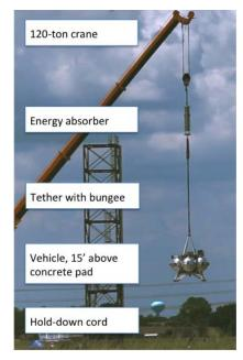
Figure 3 – Morpheus 1.5B in Tether Test Configuration
