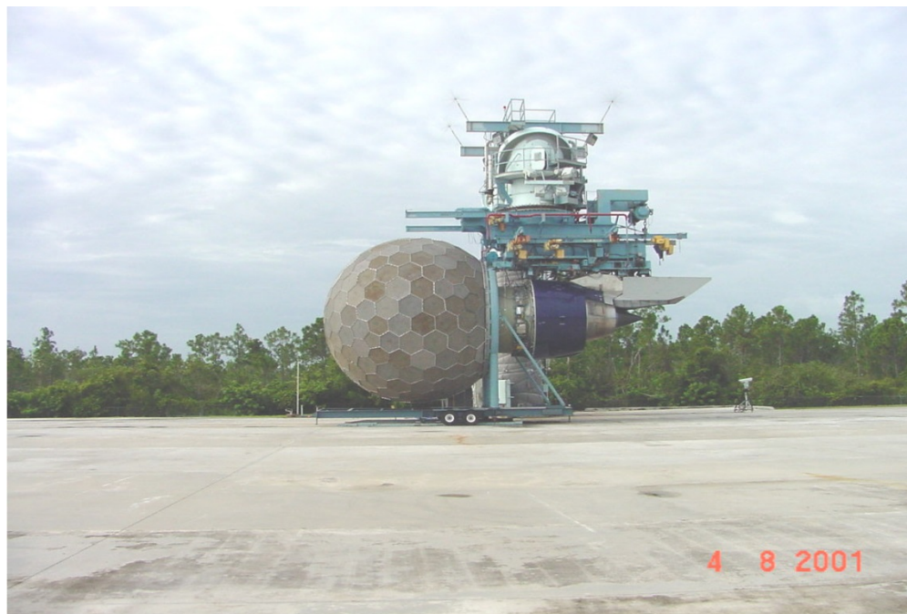
Figure 22.—PW4098 test engine with production flight inlet and ICD.
