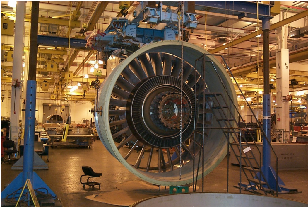
Figure 4.—The 28 vane FEGV with outer case.
