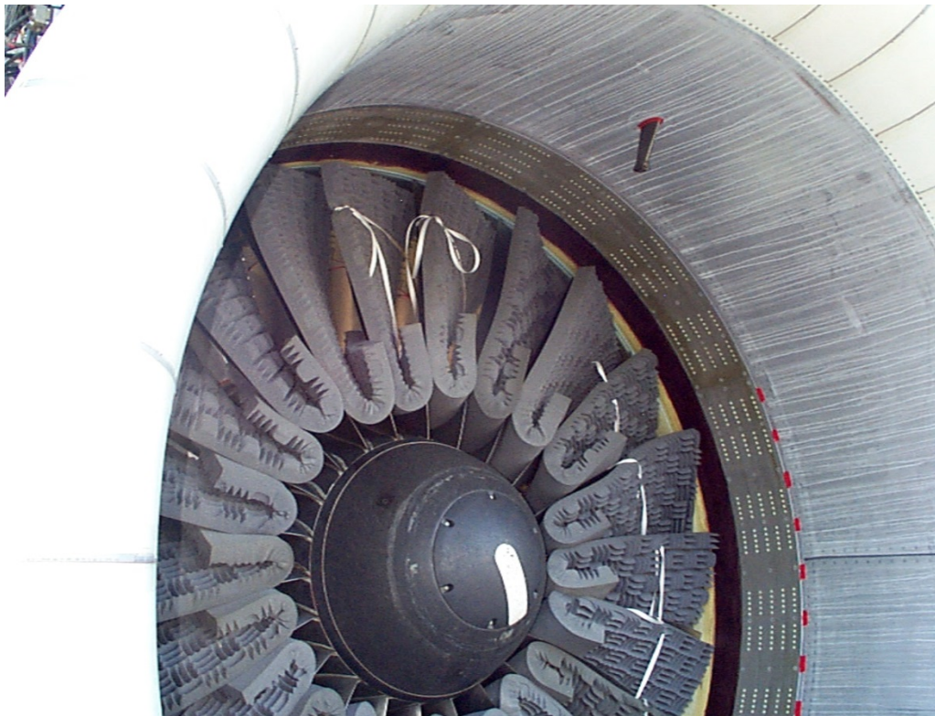
Figure 195.—Foam attached to fan blades during no flow test.
