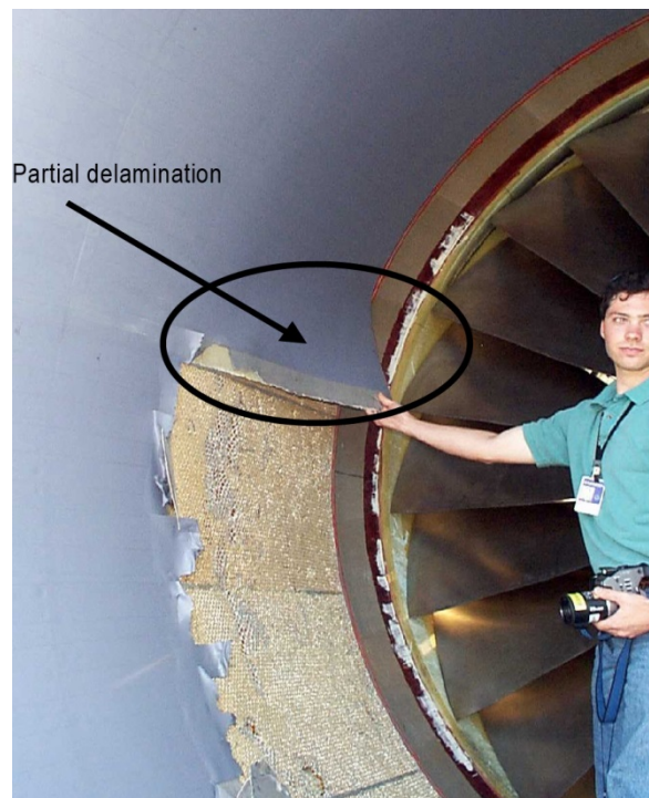
Figure 239.—Scarf inlet face sheet delamination—View 2.
