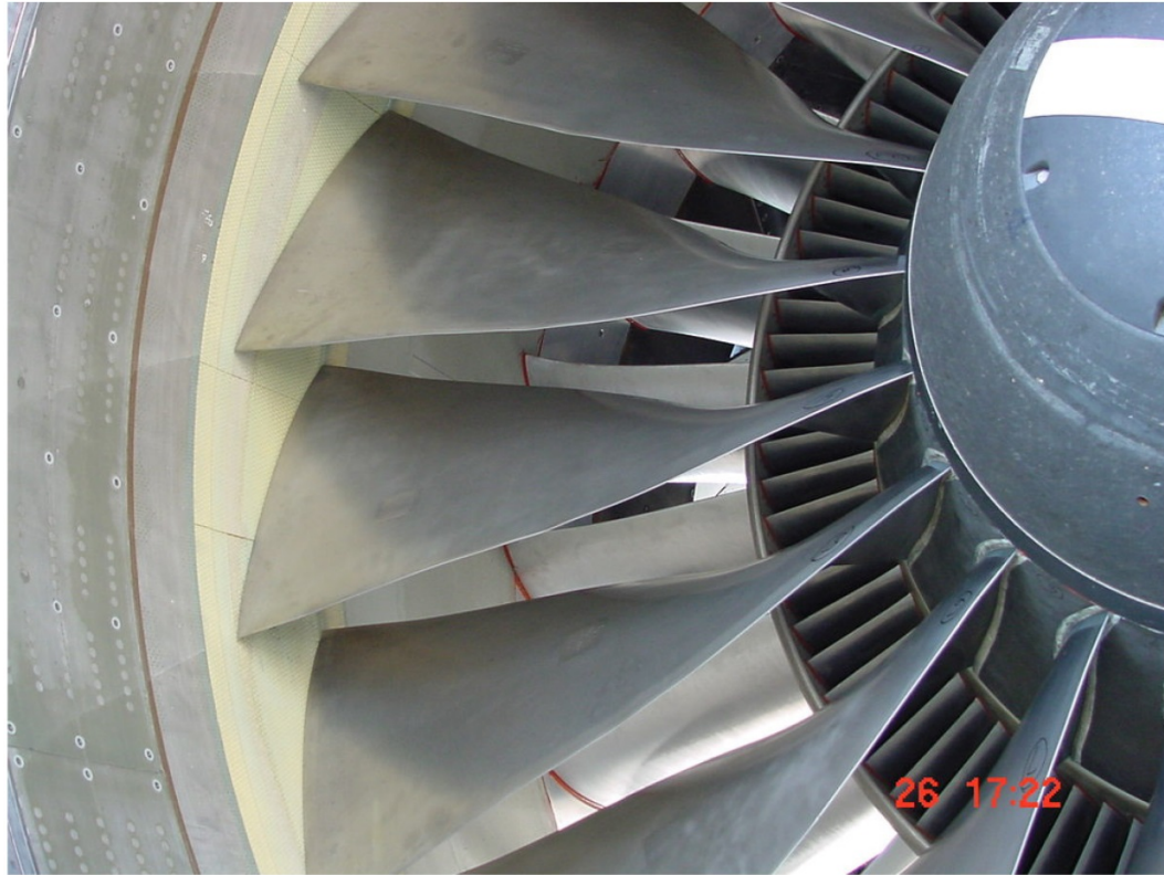
Figure 17.—Photo of 22 fan blades with 28 "cuton" FEGVs.
