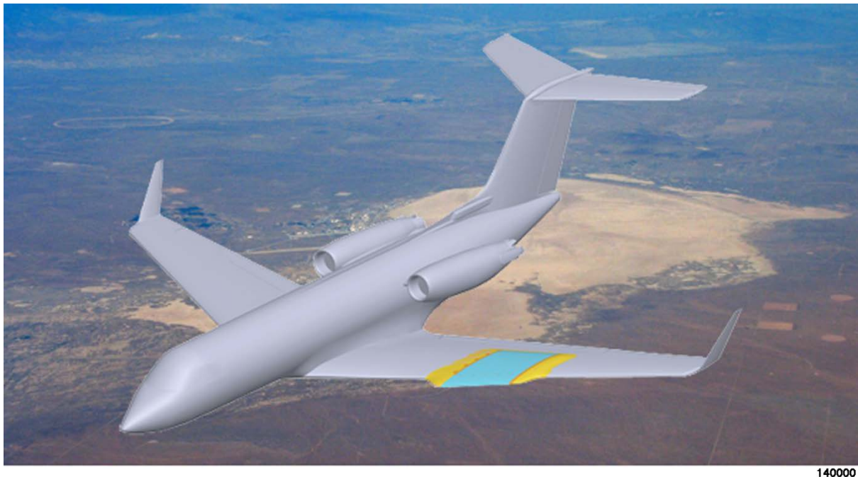
Figure 2. Conceptual sketch of the SARGE DRE laminar-flow wing glove mounted on the NASA Dryden SCRAT aircraft's left wing.
