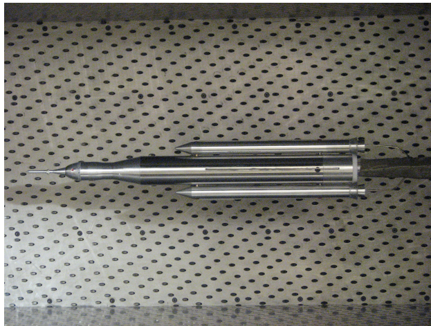
Figure 3. Force & Moment Aerodynamics Testing in the Marshall Space Flight Center 14 in. Tri-Sonic Wind Tunnel
