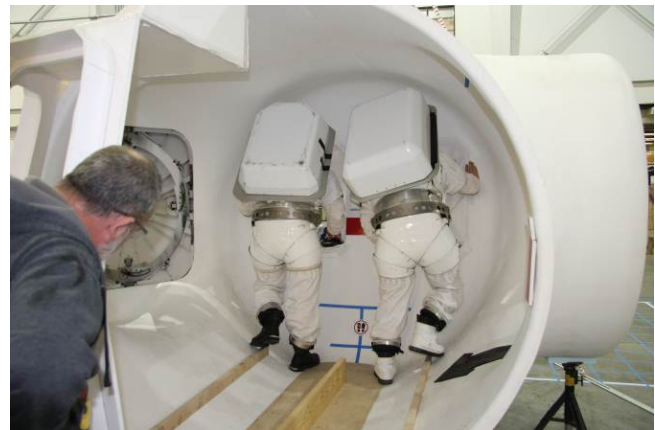
Figure 14. Mockup AAMSEV with Sub Floor
