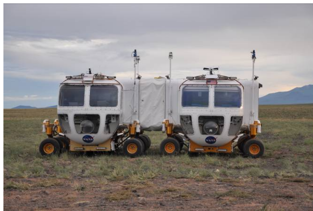
Figure 2. Two LER Cabins Docked During Desert Testing
