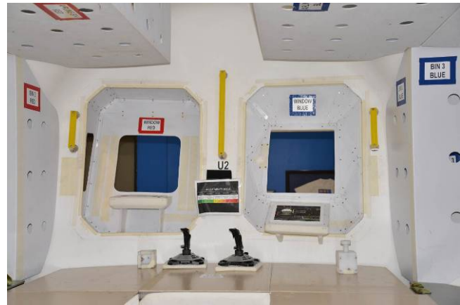
Figure 16. Integration of Red and Blue DCWUs into the AMMSEV Suit Ports
