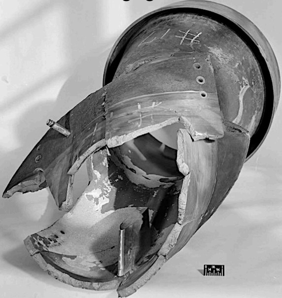
Rocket Combustion Chamber Failure During Ignition Start
