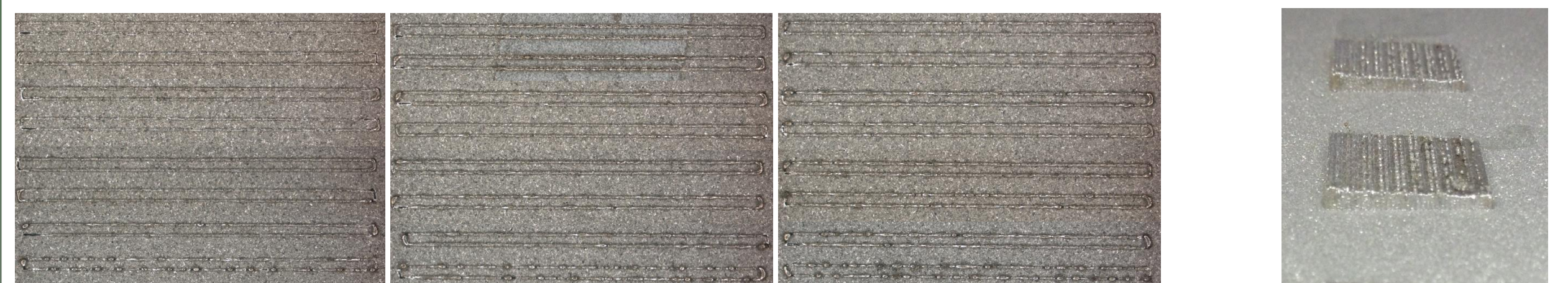
Fig 4: Single Tracks on SS Build Plate with 1, 2, 3 layers of In718 Powder
