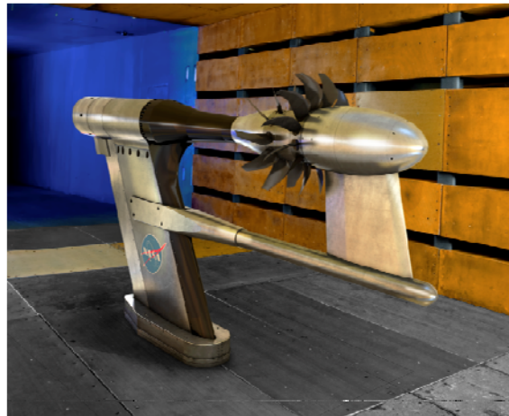
Figure 10. Illustration of the NASA Glenn Open Rotor Propulsion Rig in a 12x10 propeller fan blade configuration in the Glenn anechoic 9'x15' Low Speed Wind Tunnel. Also shown in the illustration is the generic engine pylon simulator and support sting installed in front of the rotors to determine installation effects on the rotor system performance.
