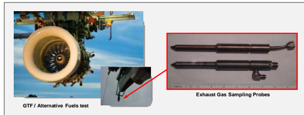
Figure 6. Geared Turbofan Demonstrator Engine shown on P&W engine test stand during Alternative Fuels test. Inset in the center shows the exhaust gas sampling configuration. Inset on the right side of the picture is a close-up view of exhaust sampling probes used during testing.
