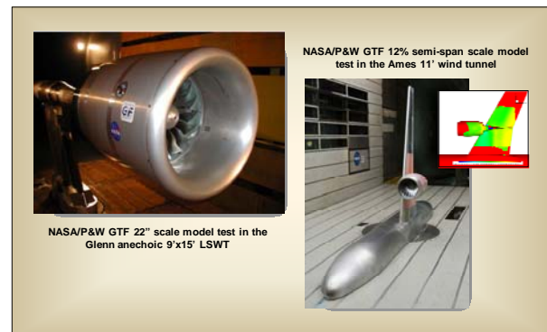
Figure 4. Highlights of NASA/P&W collaborative, scale model tests of the Geared Turbofan.
