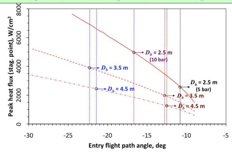
2.5 m dia. case has high peak heat flux *and* pressure at steepest entry Heat fluxes greater than 2.5 kW/cm<sup>2</sup> are hard to achieve in current arc jets
