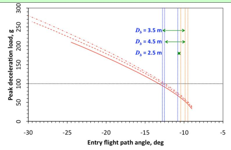
Very narrow (< 0.5°) entry flight path angle window for highest ballistic coeff.
