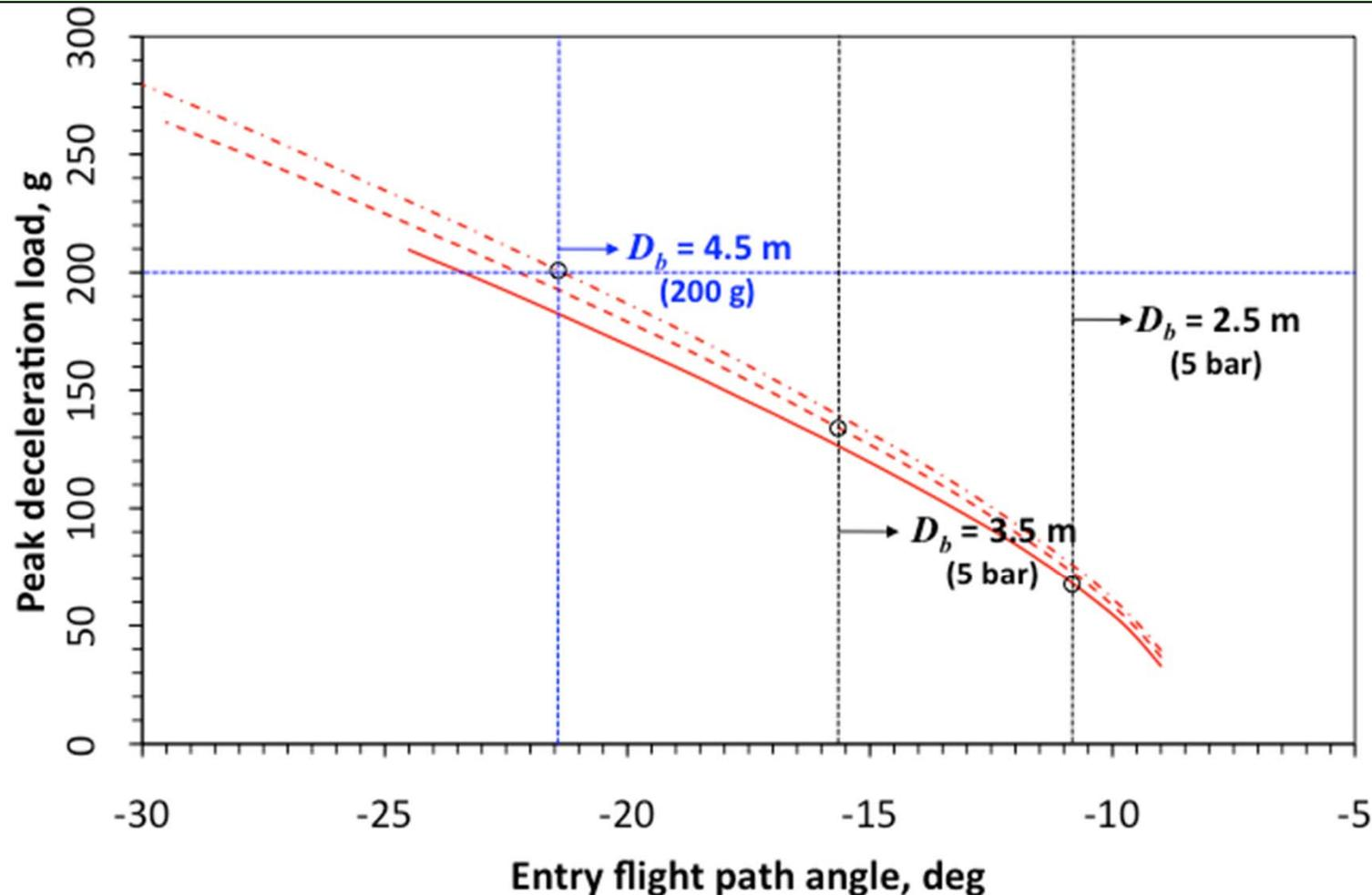
For 2.5 m and 3.5 dia., steepest entry is determined by the pressure limit (10 bar)
