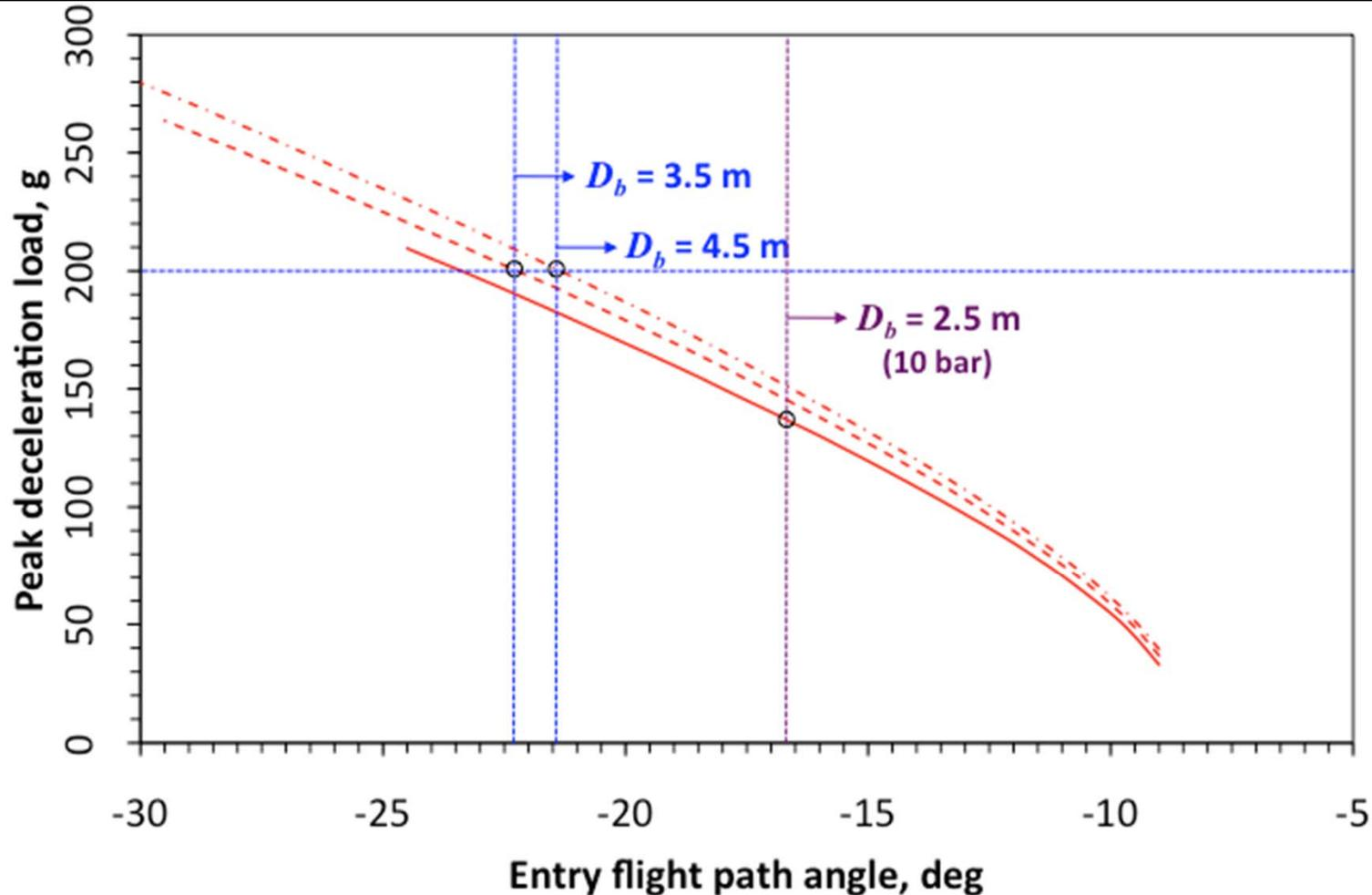
For 2.5 m dia., steepest entry is determined by the pressure limit (10 bar)
