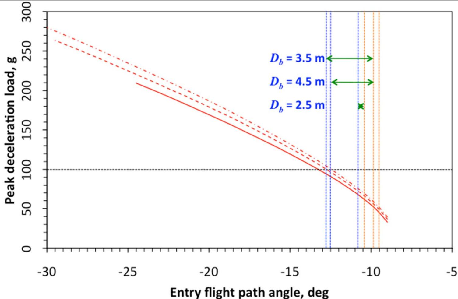
Very narrow ( $< 0.5^\circ$ ) entry flight path angle window for highest ballistic coeff.
