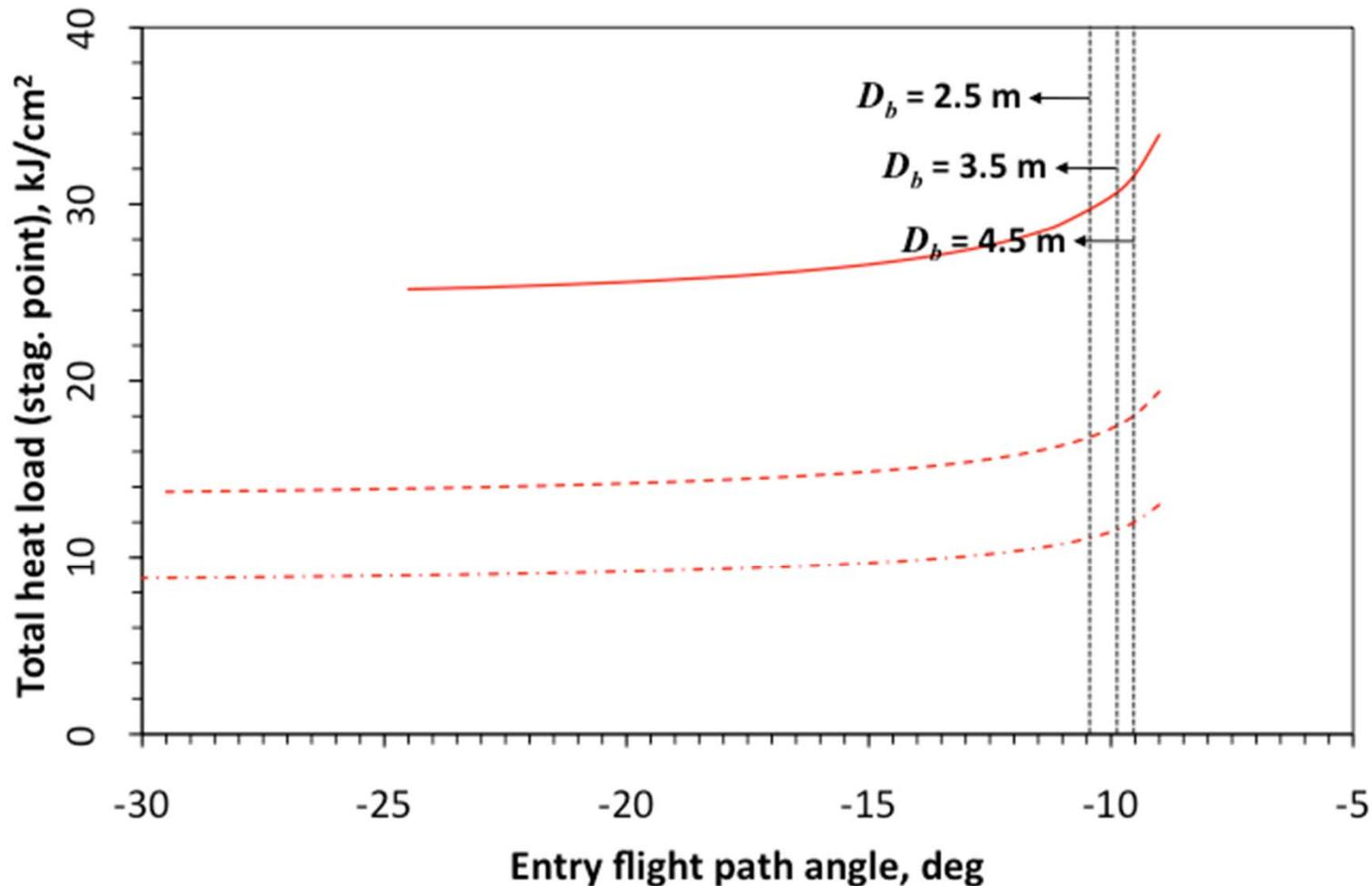
Entry angles correspond to max. curvature in heat load curves for highest  $\beta_E$
