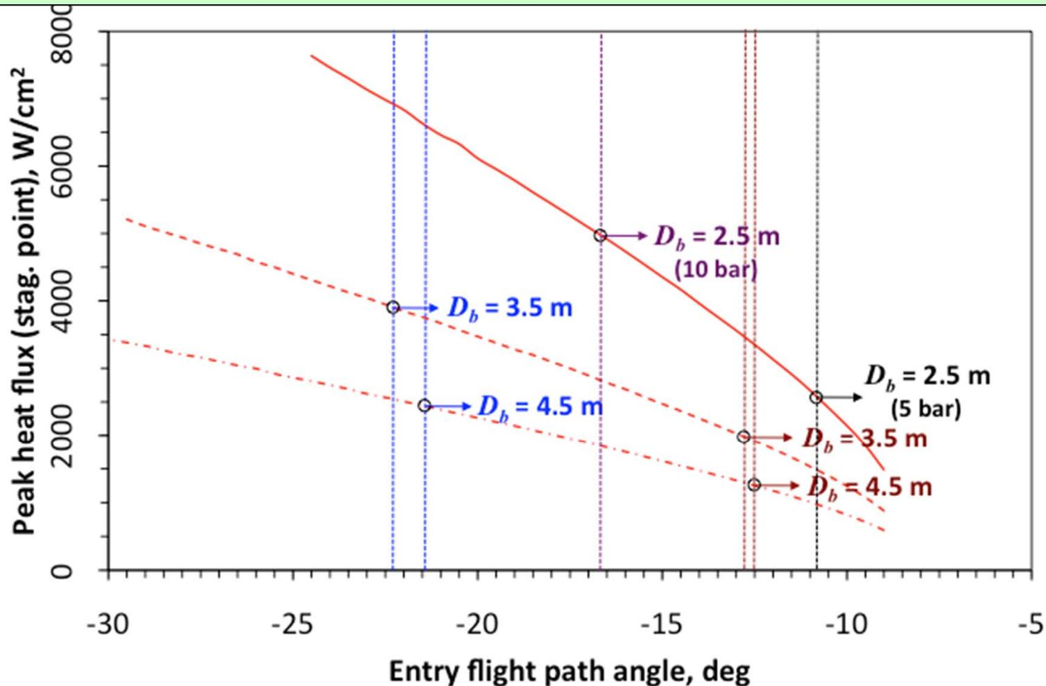
2.5 m dia. case has high peak heat flux *and* pressure at steepest entry
