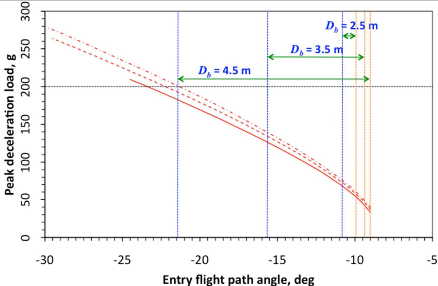
Pressure load limit still limits entry flight path angle window for highest ballistic coefficient
