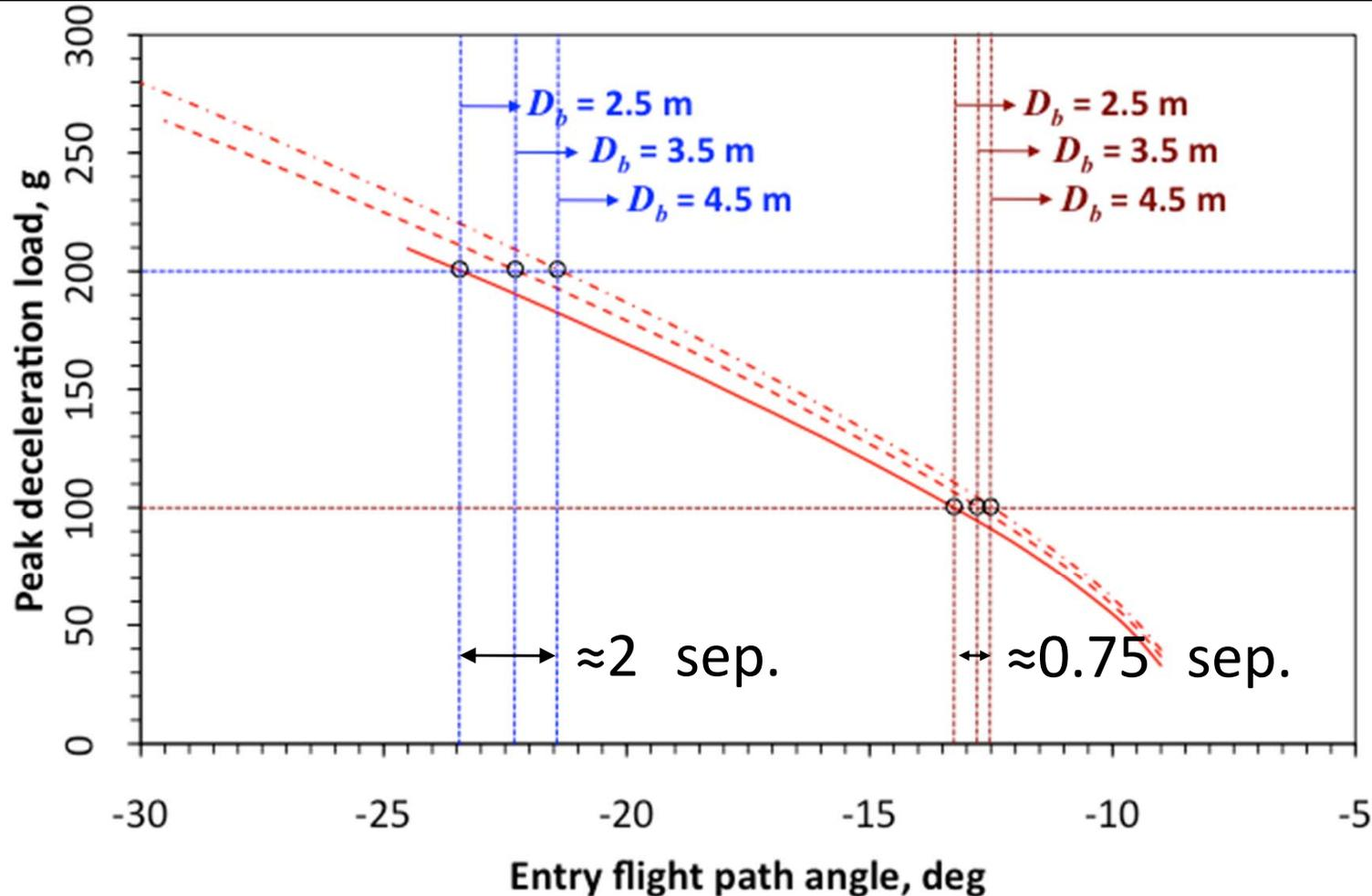
Separation between ballistic coefficients increases with increasing g load limit
