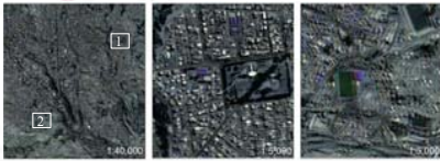
Figure 1. Training site for the mountainous city of Nuestra Señora de La Paz, Bolivia with original image overlaying orthorectified image at 60% transparency. Note the difference between sections 1 and 2 of the training site. The orthorectification process made significant adjustments to section 2 which lies lower in the mountain valley.
