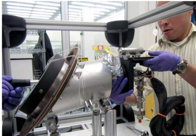
Figure 2: Technicians work on an MR-104G thruster, in preparation for the Orion Propulsion System Hot Fire Test.
