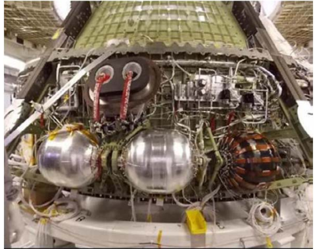
Figure 3: Orion EFT-1 Crew Module Midway Through Propulsion Installation. http://www.nasa.gov/sites/default/files/files/OrionMARAugust2013.pdf
