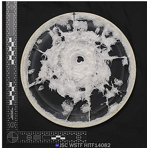
Figure 1, Complete penetration of fused silica pane.
