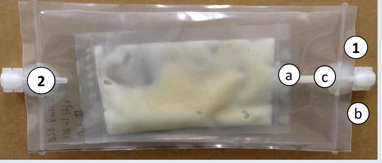
or FDA approved Masterbond EP21LV (Hackensack, NJ) for suited tests, was used to connect tubing and adapters. (2) Septum adapter assembly sealed into outer pouch for connection of tubing from outer pouch to pontube.
