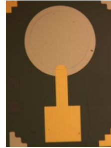
Fig. 2. a) Schottky diode with contact pad fabrication process. b). Image of a Pd/PdO x /SiC diode with a Au/Ti contact pad. The dark area surrounding the sensor-pad is SiO 2
