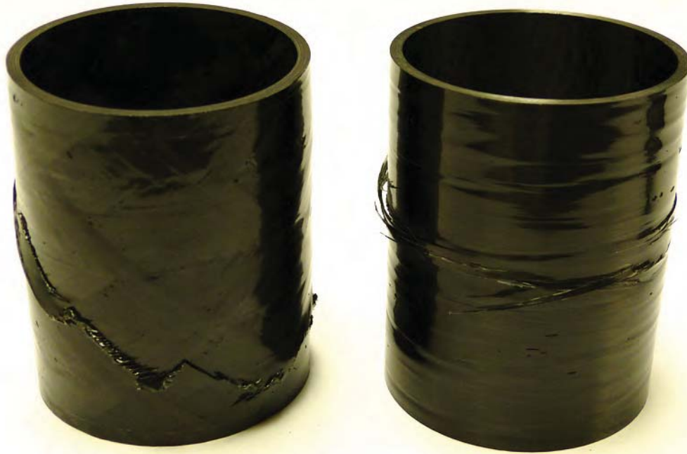
Figure 25.—Examples of compression specimen failures, \pm 45 (left) and 90 (right).
