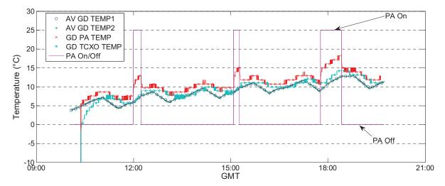
Figure 4.—Temperature increase when the SDR is transmitting (November 2, 2012).
