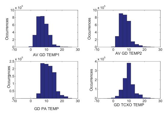
Figure 1.—GD SDR temperature histograms.
