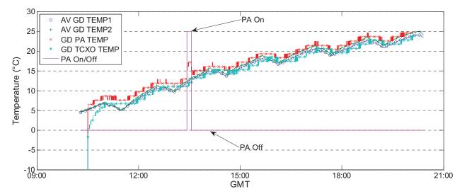
Figure 3.—GD SDR temperature after power on (November 6, 2012).
