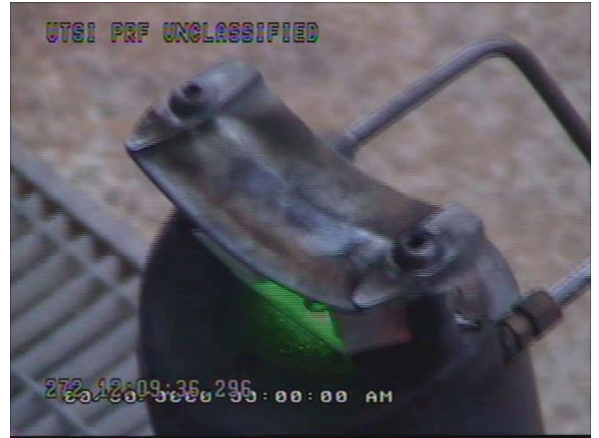
Overhead View of Vane in Afterburner Flame
