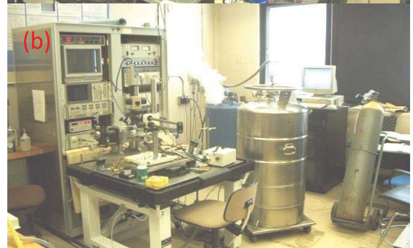
(a) 40 GHz Cryogenic On-Wafer Probe Station; (b) 2.5 K, 9 T Hall system
