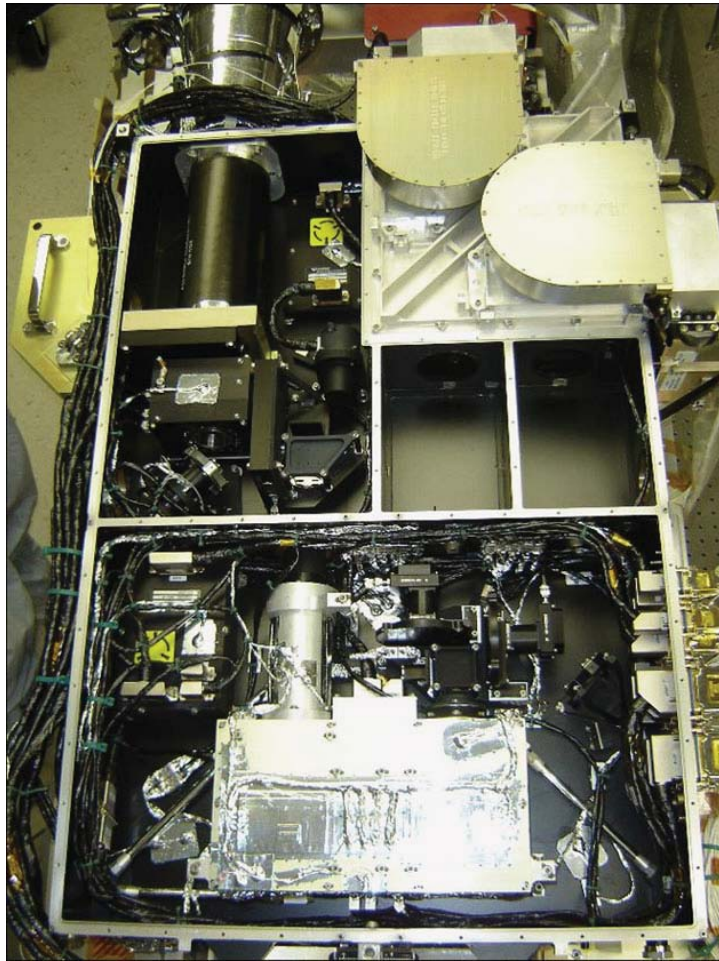
Figure 2 Photograph of the inside of the optics package. Light enters through the telescope at the upper left, passes through the chain of filters near the bottom, and is detected by the CCD cameras at the upper right. The box is roughly 88 cm long by 55 cm wide by 16 cm high. The various elements are identified in Figure 1.
