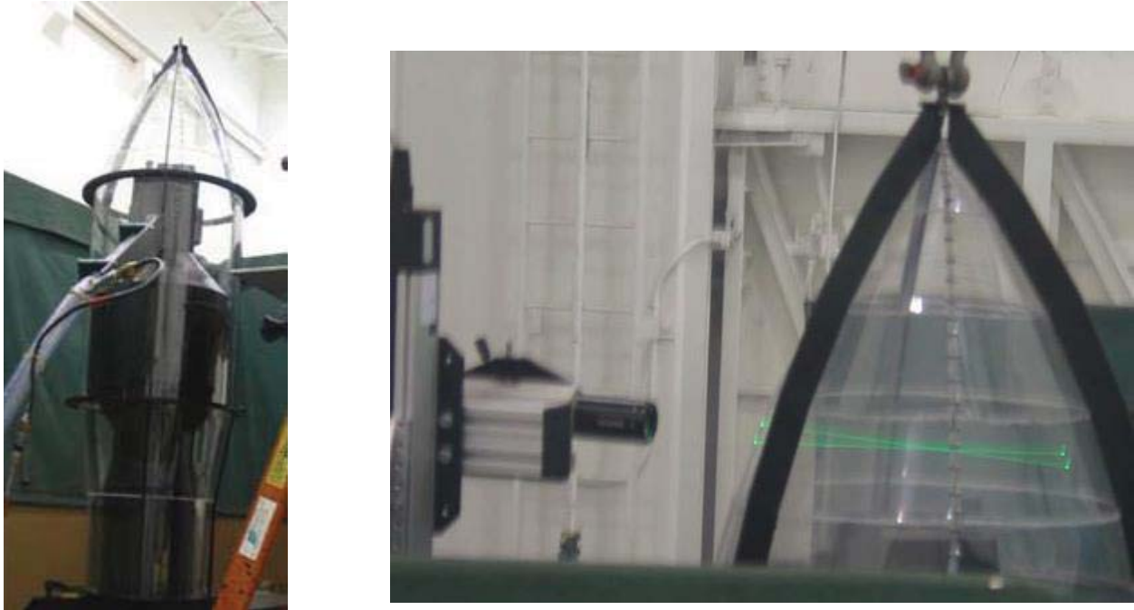
Figure 16: Environmental Control System (ECS) Airflow Testing [24]
