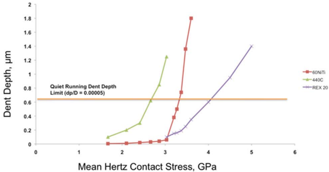
Figure 1. Dent Depth Versus Mean Contact Stress for 12.7 mm Diameter \text{Si}_3\text{N}_4 Ball Pressed Onto Flat Plate Specimens.
